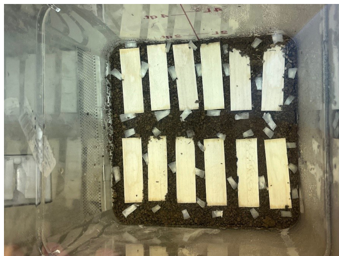
Figure 2. An 8-L soil block container with 12 aspen feeder strips inoculated with mycelial plugs of the white-rot fungus, Irpex lacteus .
