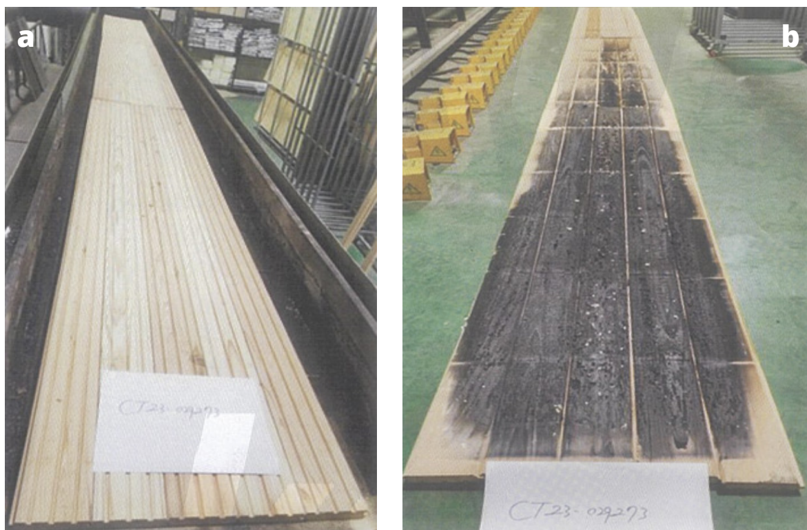
Figure 4. Photographs of cedar siding specimens before (a) and after (b) Steiner tunnel testing.
