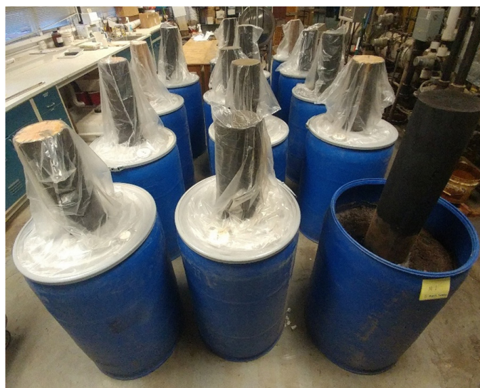
Figure 1. Photo of post-in-barrel test showing southern pine and Douglas-fir posts set in soil within plastic drums. Posts were covered with plastic sheeting to prevent dust from accumulating on the surface, and one pine post is shown uncovered just before sampling.
