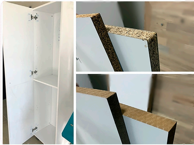
Figure 1. Examples of the test shelves along with side views of the MDF and PB shelves.
