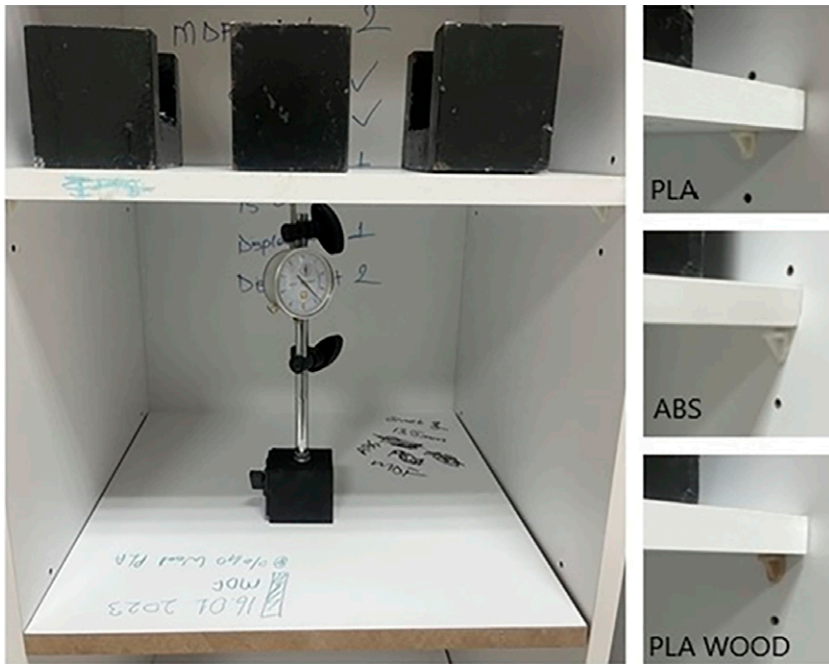
Figure 8. Photos showing the loads applied to a shelf unit as well as examples of shelves with the three-pin materials.
