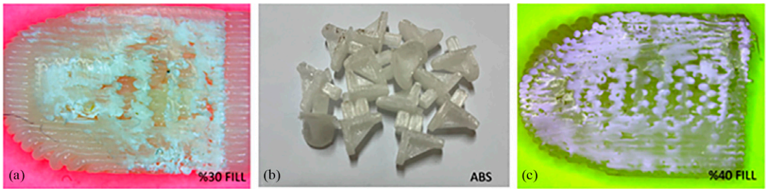
Figure 4. Examples of (b) ABS filament pins along with microscopic images of pins with 30% or 40% fill ratios (a and c, respectively).
