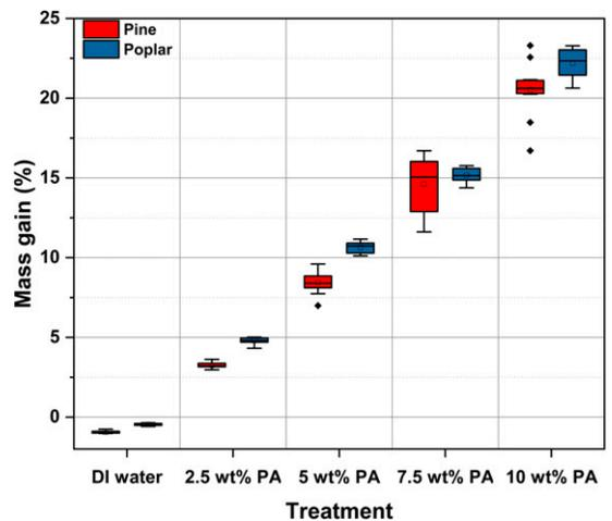
Figure 2. Mass gain of wood blocks after treatment.
