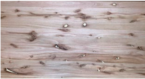
F 6 : 6 mm thick fibre E. nitens glued to marine ply substrate and veneer backing
