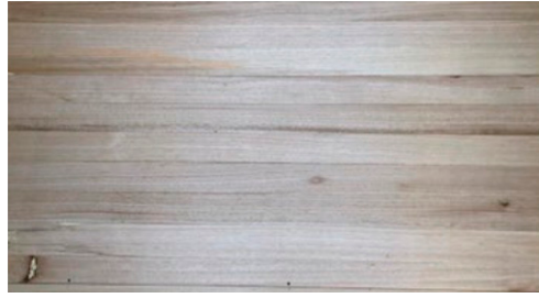
S 6b : 6 mm thick sawlog E. nitens glued to marine ply substrate
