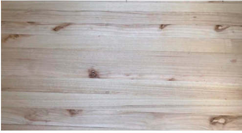
S 6a : 6 mm thick sawlog E. nitens glued to marine ply substrate and veneer backing
