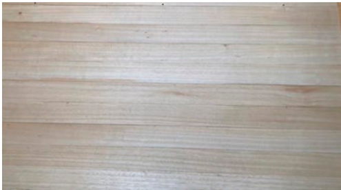
S 1.2mp : 1.2 mm thick sawlog E. nitens glued to marine ply substrate and veneer backing
