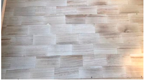
D 12 : 12 mm thick solid, densified E. nitens
