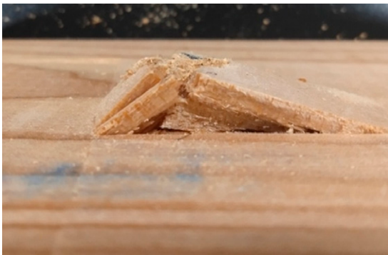
Figure 11. Typical withdrawal failure mode.
