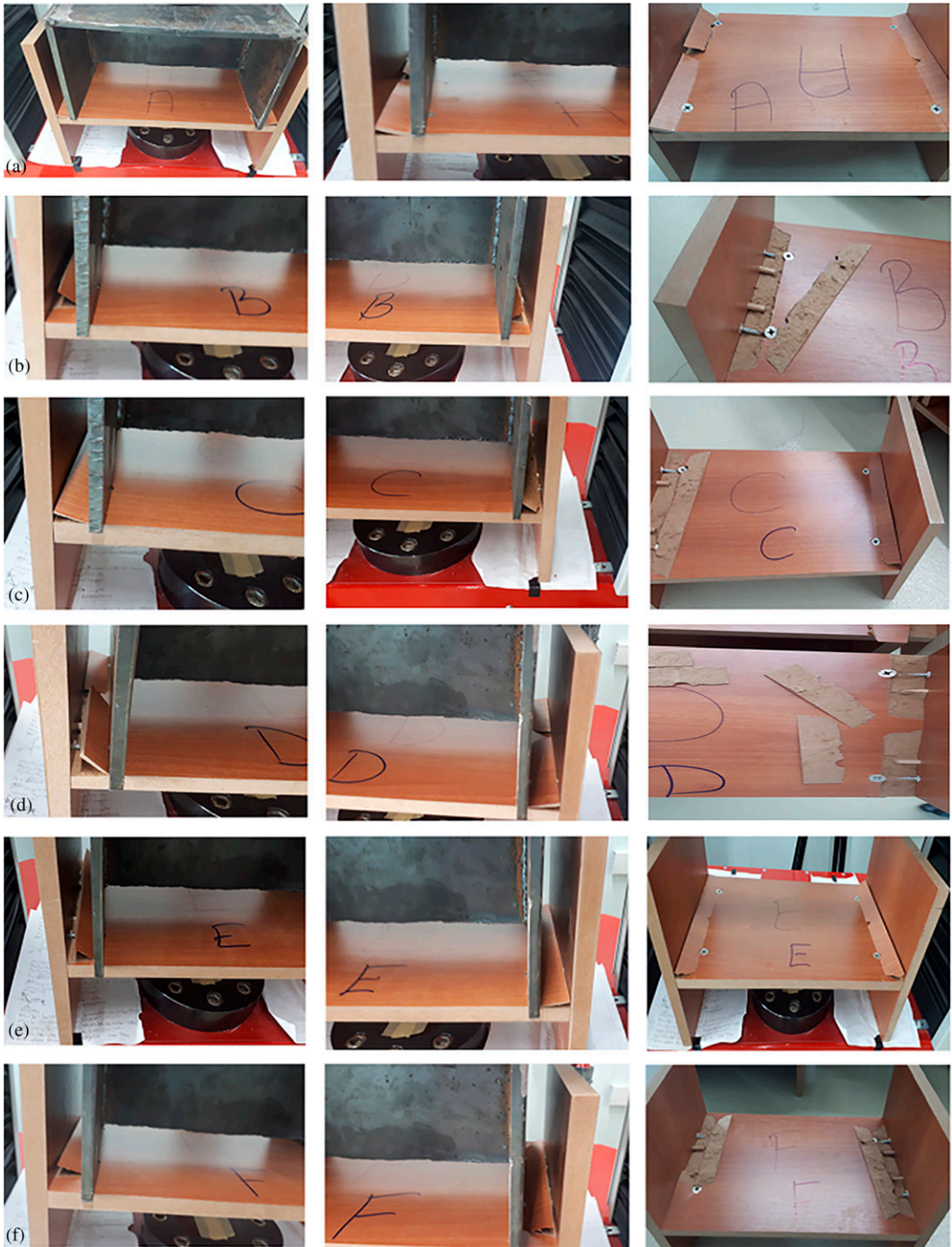
Figure 4. Types of deformation of H-type furniture joints resulting from the compression test: 54 mm end distance + oak dowel (a), 90 mm end distance + oak dowel (b), 72 mm end distance + oak dowel (c), 54 mm end distance + beech dowel (d), 72 mm end distance + beech dowel (e), and 90 mm end distance + beech dowel (f).
