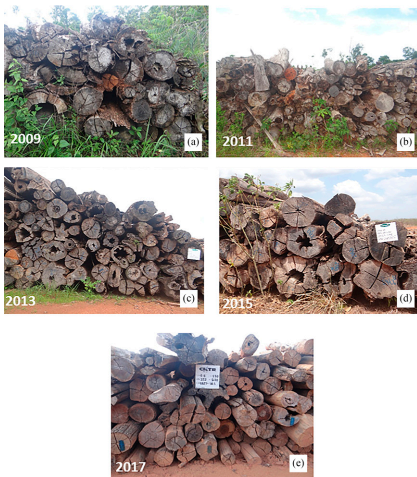
Figure 1. Logs piling under different periods of exposure: (a) 8 yr; (b) 6 yr; (c) 4 yr; (d) 2 yr; and (e) 0 yr of exposure.
