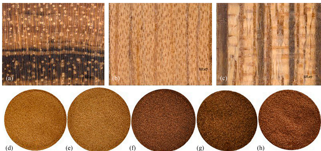
Figure 8. Macroscopic images of Astronium lecointei (a-c: cross-section, tangential, and radial, respectively); variation in color due to storage times from 0 to 8 yr (d-h, 0, 2, 4, 6, and 8 storage years, respectively).
