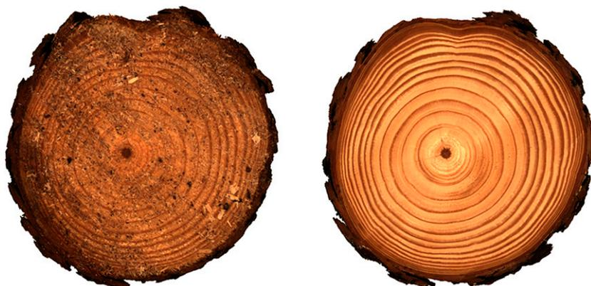
Figure 2. The left image shows the typical surface quality of a chainsaw-cut wood disk; the right image shows the same disk after surface preparation (background removed from both images).
