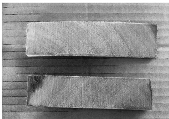
Figure 5. Example of extremely shallow and minimal penetration in the heartwood of conventional vacuum pressure treated E. nitens as indicated by darkened color on the corners of samples sprayed with PAN (1-[2-pyridylazo]-2-naphthol) for the presence of copper.
