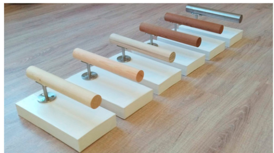
Figure 1. Handrail samples (from left to right: unmodified spruce, unmodified pine, acetylated radiata pine, thermally modified pine, thermally modified spruce, stainless steel).
