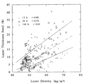
FIG. 7. The relationship between layer density and layer thickness swell of the oriented strandboard.
