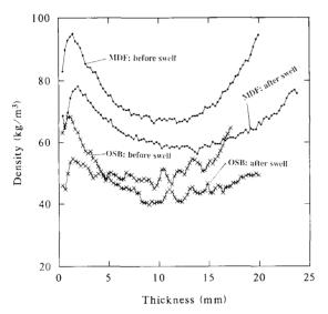
FIG. 5. Vertical density distributions of the medium density fiberboard and oriented strandboard before and after water soak for 168 h.
