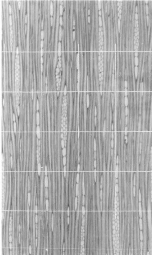
FIG. 2. A twenty-five-point grid superimposed over a tangential-longitudinal wood section. The grid lines are oriented perpendicular and parallel to the long axis of the rays.
