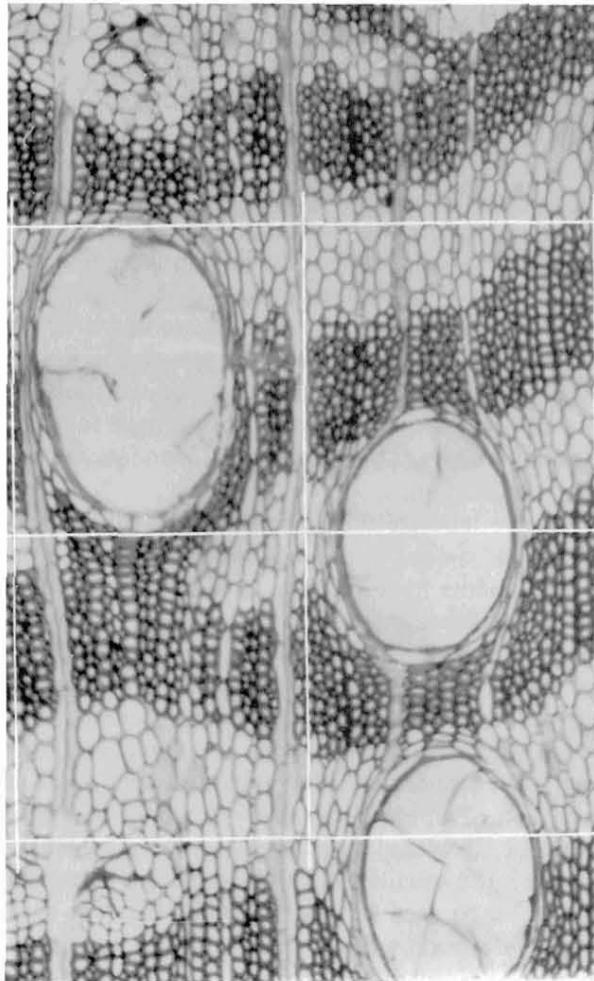
FIG. 1. A nine-point grid superimposed over the transverse section of a diffuse porous wood. Note that the grid lines are oriented parallel and perpendicular to the rays.
