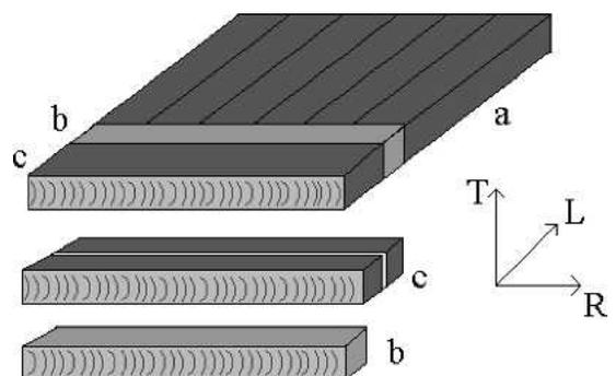
FIG. 1. Preparation of specimens for a) mechanical features, b) anatomical characteristics and c) densitometry.
