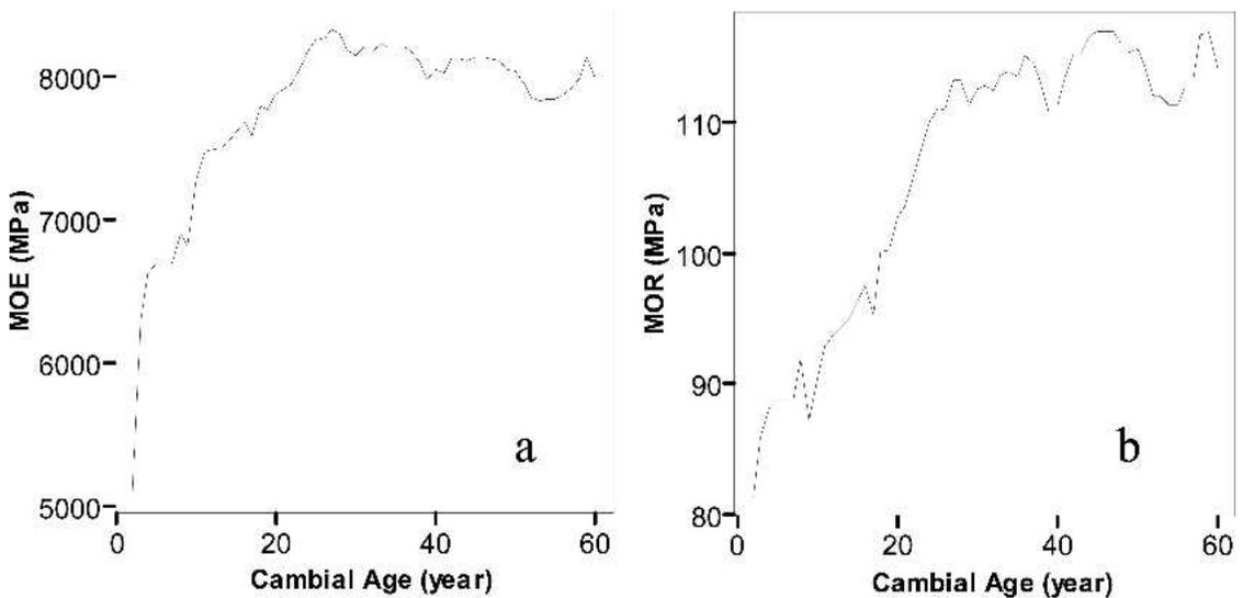
FIG. 2. Radial variation (measurement averages) from pith to bark of a) MOE and b) MOR as a function of cambial age.
