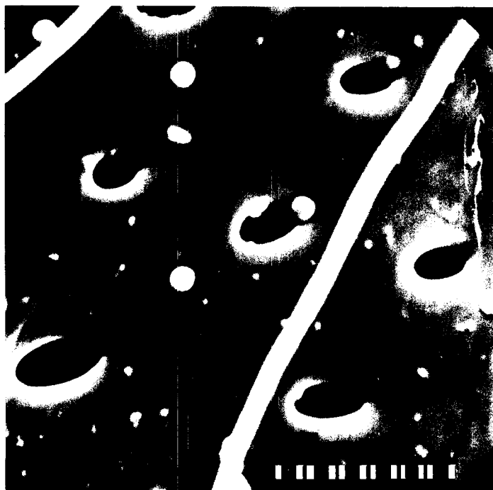
FIG. 1. Tangential intervessel pits of black cherry ( Prunus Serotina EHRH) carbonized to 900 C showing latex beads used for calibration.
