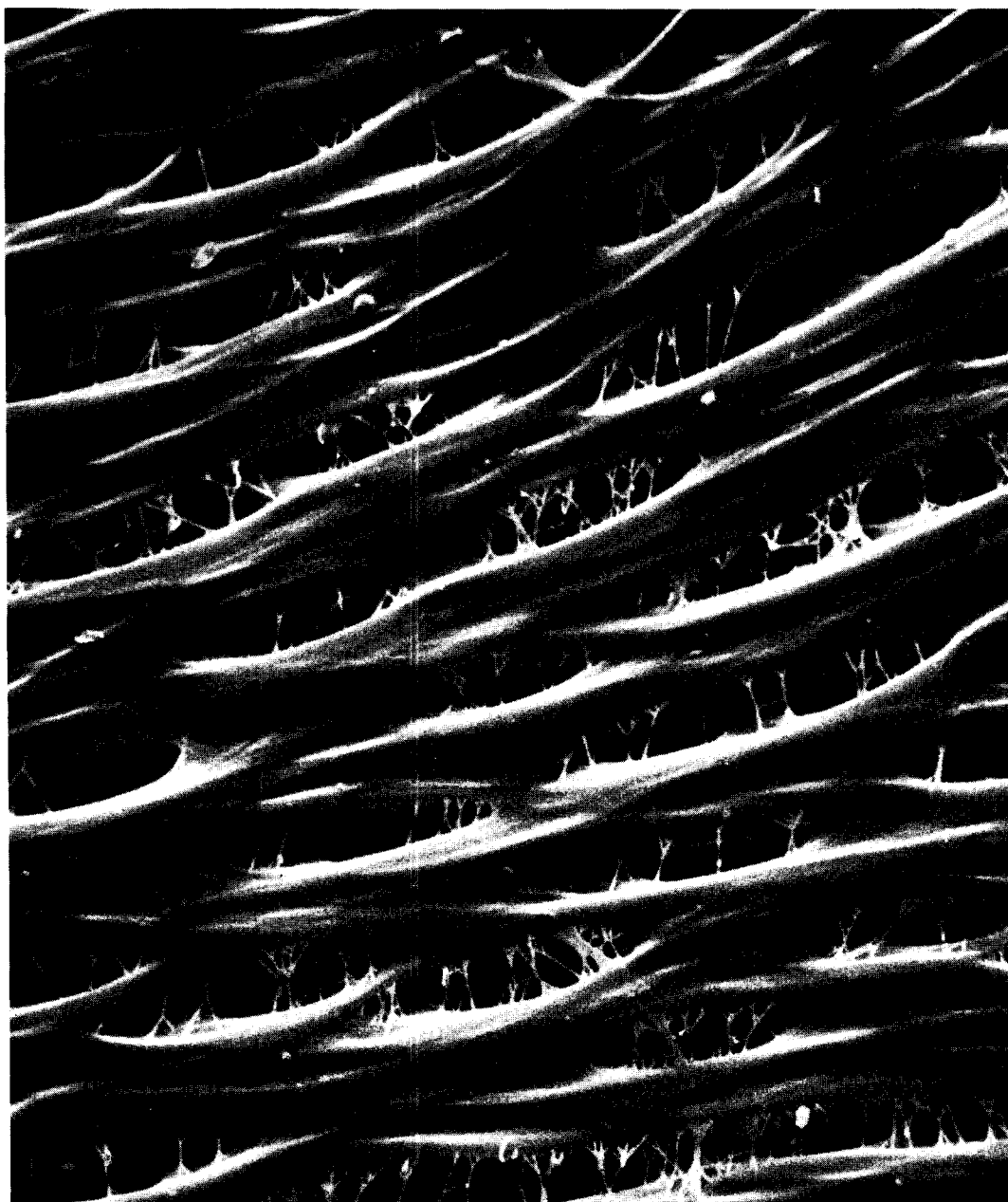
FIG. 5. Microfibrillar webs traversing the vessel pit apertures in Corynocarpus laevigatus (air-dried, hypochlorite-treated). \times 4,500 .
