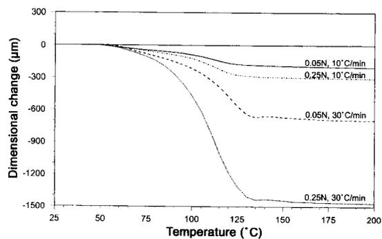
FIG. 4. Thermo-mechanical analysis profiles for powdered resin determined using different heating rates and applied pressures.
