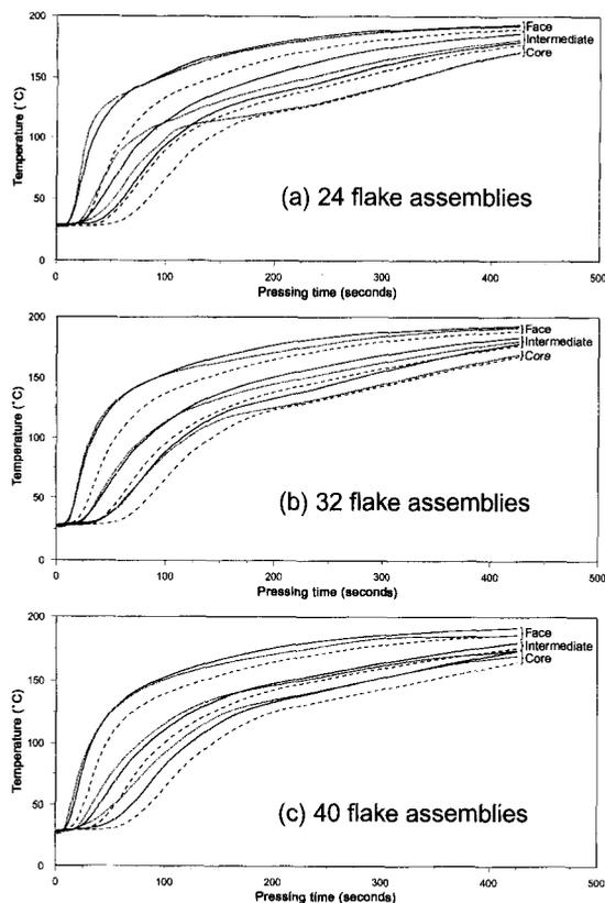
FIG. 2. Temperatures recorded at different layers during hot-pressing of flake assemblies made from different numbers of flakes (— 15 seconds press closing time, 4.5% moisture content; --- 45 seconds press closing time, 4.5% moisture content; ..... 15 seconds press closing time, 15.5% moisture content face, 4.5% moisture content core).
