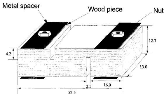
FIG. 1. Flake assembly prepared for strength test of intermediate layer. Dimensions are in mm.
