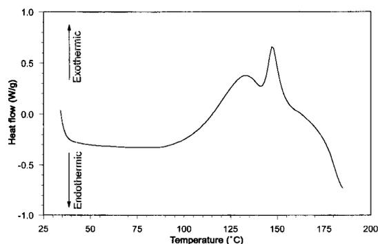
FIG. 5. Differential scanning calorimetry profile of powdered resin.
