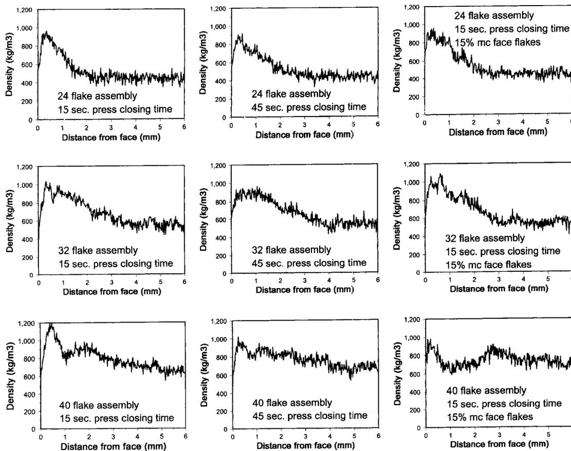
FIG. 3. Vertical density distributions determined for flake assemblies produced using different numbers of flakes and pressed at different press closing times. All flakes at 4.5% moisture content unless otherwise indicated. Each distribution shown represents the average of two face-to-core measurements for each of three replications (i.e., six face-to-core measurements).
