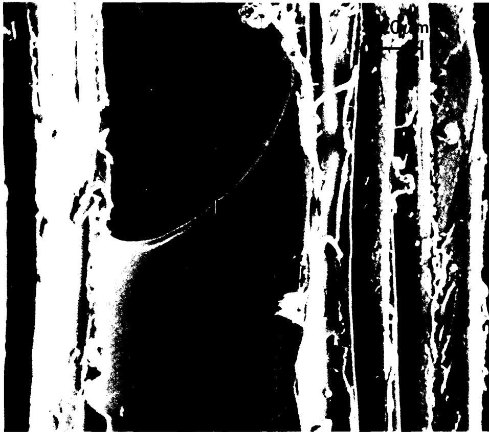
FIG. 2. A single vessel element end in the sapwood of aspen. The end, seen as the diagonal in the photomicrograph, protrudes from the vessel element wall but does not close the vessel.
