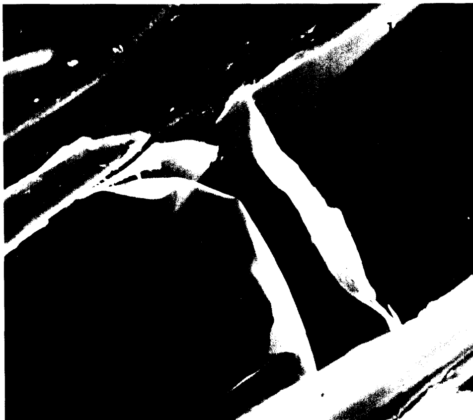
FIG. 5. Two tyloses in a single vessel of aspen heartwood. Pits in the vessel wall are visible between the tyloses.
