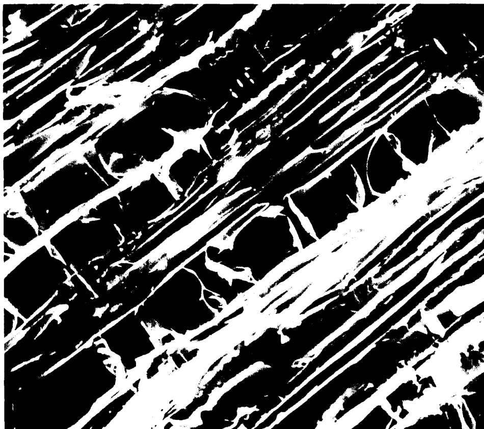
FIG. 3. Aspen heartwood showing numerous tyloses closing the vessels.
