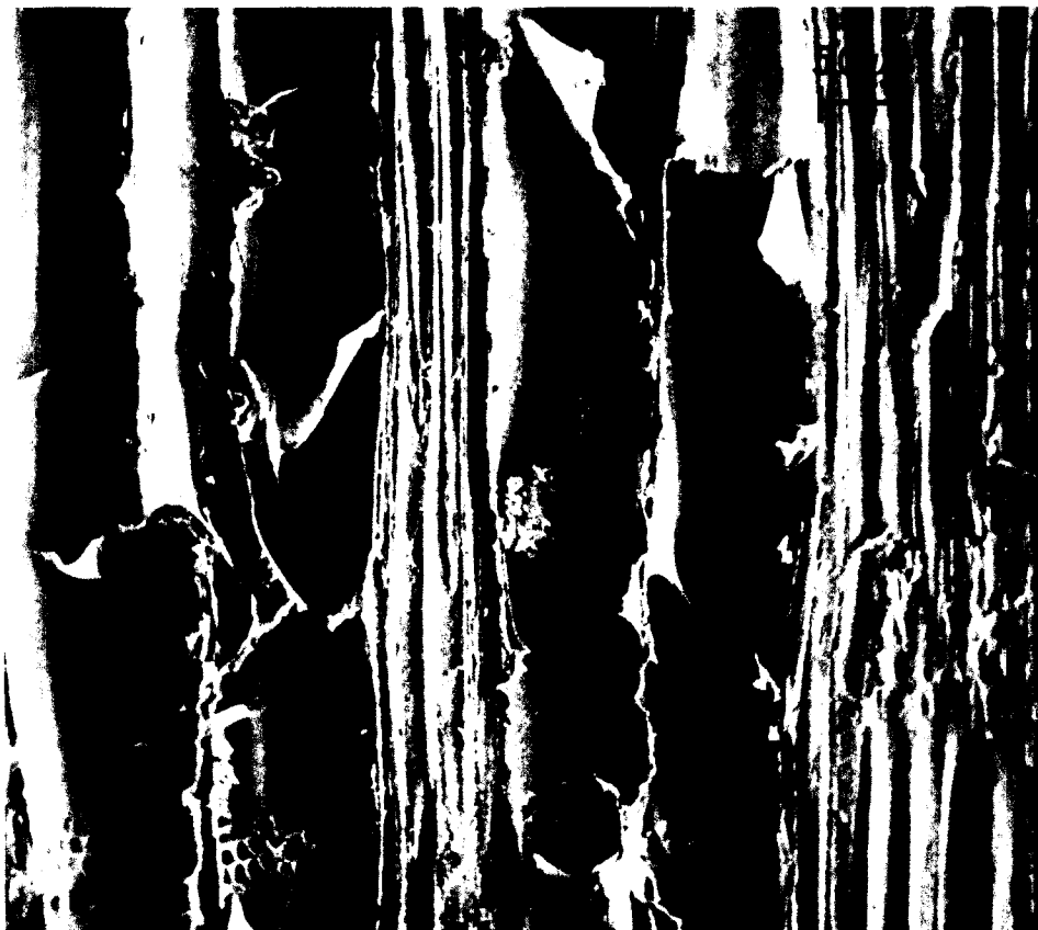
FIG. 1. Aspen sapwood with diagonal vessel element ends projecting from the lumen walls and some pitting in the walls. Except for these wall sculpturings, the vessels are open for fluid transport.
