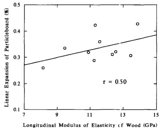
FIG. 3. Simulated linear expansion of particleboard in relation to longitudinal modulus of elasticity of wood.
