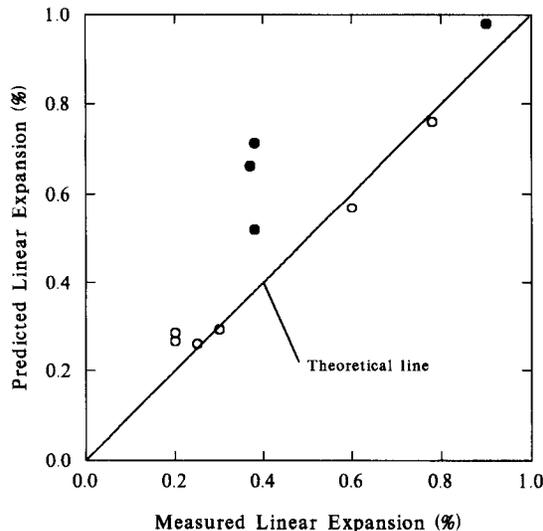
FIG. 8. Comparison of measured linear expansion and model predicted linear expansion. The measured values were read from the figures of corresponding literature and were the average if more than one board condition was involved. The filled symbols indicate that an upper relative humidity of 90% was used. The open symbols indicate that an upper relative humidity less than or equal to 80% was used.
