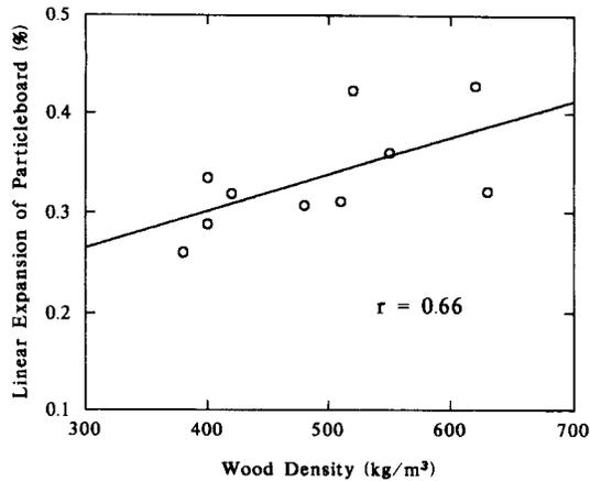
FIG. 4. Simulated linear expansion of particleboard in relation to wood density.
