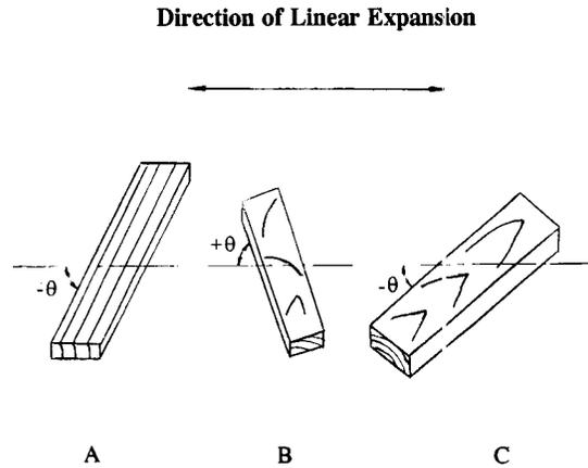
FIG. 1. A schematic showing the definition of particle configuration and orientation angle relative to the direction of linear expansion. A = longitudinal-radial (L-R) configuration; B = intermediate configuration; C = longitudinal-tangential (L-T) configuration.
