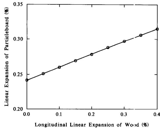
FIG. 5. Simulated linear expansion of particleboard in relation to longitudinal linear expansion of wood (wood species: quaking aspen).
