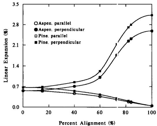
FIG. 7. Simulated linear expansion of aspen and southern pine single-layer oriented strandboard to percent alignment of particles in the orientation and across the orientation directions.
