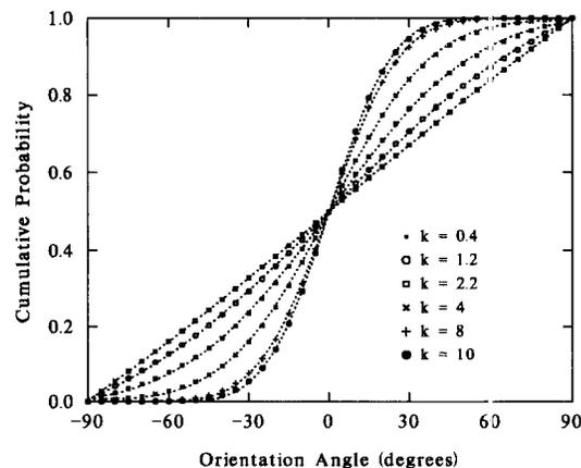
FIG. 6. Influence of concentration parameter ( $k$ ) on the cumulative probability distribution of the orientation angle.
