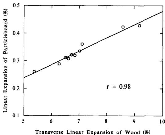
FIG. 2. Simulated linear expansion of particleboard in relation to transverse linear expansion of wood.
