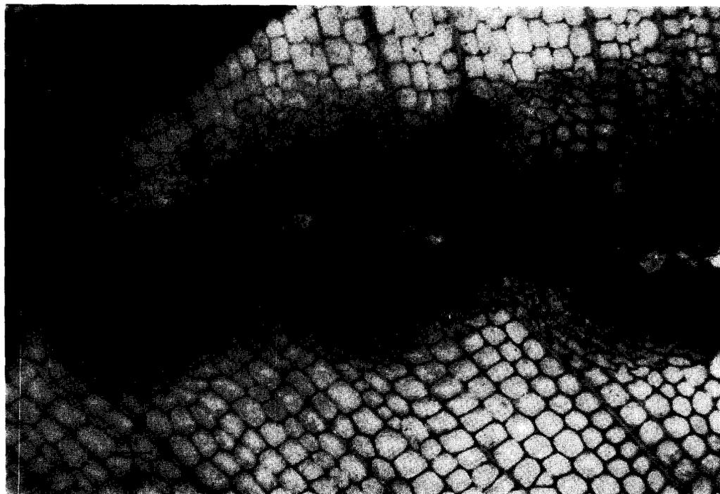
FIG. 2.—Photomicrograph of glueline in Douglas-fir abrasively planed with 36-grit open coat aluminum oxide ( $170\times$ ). Crushing and distortion of cells are evident near glueline. (M 144 038)
