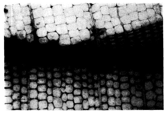
FIG. 3.—Photomicrograph of glueline in knife-planed and laminated Douglas-fir  $(290 \times)$ . Cells near glueline are clean-cut, with little crushing or distortion. (M 144 037)
