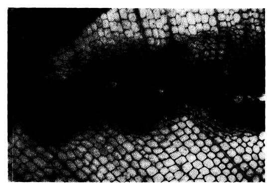
FIG. 2.—Photomicrograph of glueline in Douglas-fir abrasively planed with 36-grit open coat aluminum oxide  $(170 \times)$ . Crushing and distortion of cells are evident near glueline. (M 144 038)
