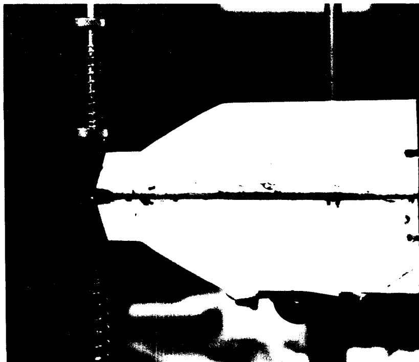
FIG. 4. Specimen mounted with knife-edged grips in preparation for cleavage test. Position of knife edge of grips corresponds to a = 0 .
