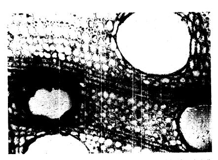
Fig. 6. Small, treated vessel surrounded by treated parenchyma and the remaining tissue including three vessels untreated in O. sumatrana heartwood.  $640 \times$ .
