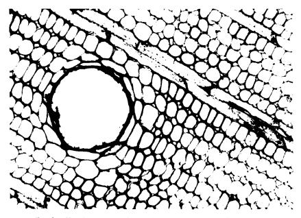
Fig. 3. H. ovigera sapwood treated vessel and all visible fibers. 640×.
