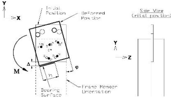
FIG. 2. Response of NPC to moment loading.
