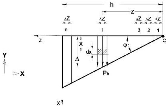
FIG. 3. Diagram of the plate bearing on the end grain.
