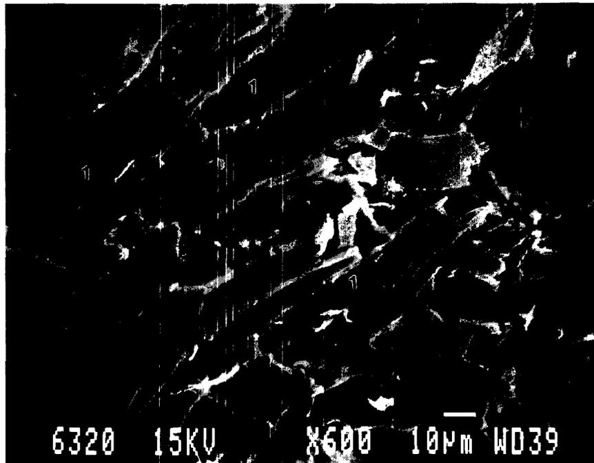
FIG. 9. A fracture surface of an internal bonding test specimen. The composite is composed of wood fibers and 5% MDI based on the total oven-dry weight of wood fibers. Fiber split occurs in the fracture surface (1).
