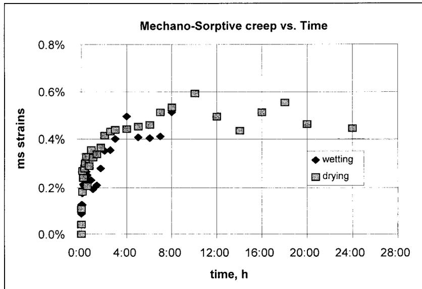
FIG. 7. Mechano-sorptive creep as it appears after subtraction of the viscoelastic strain components.
