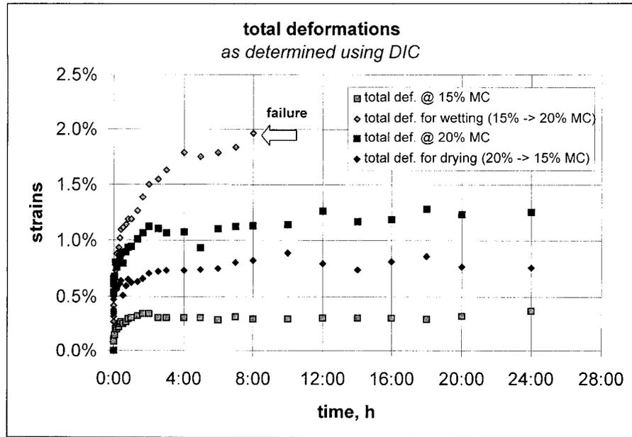
FIG. 5. Total deformations recorded during the creep tests with constant and changing MC, determined using DIC. Points are determined as averages of points determined for all specimens undergoing the same MC regime for the same time.
