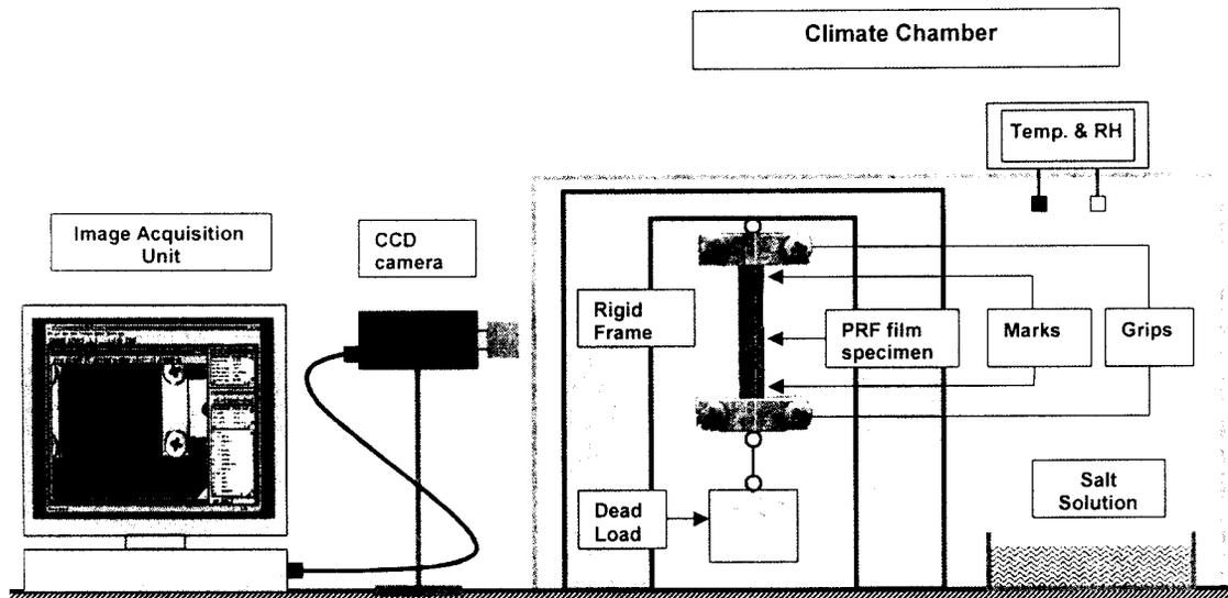
FIG. 3. Schematic of the experimental setup for the creep tests. In free shrinkage and swelling tests, additionally a sensitive balance was added to trace MC changes.
