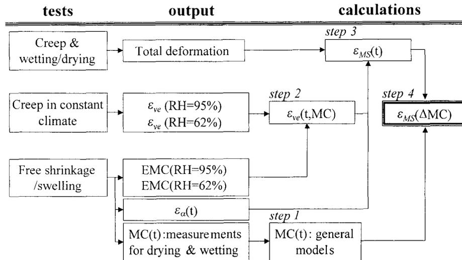
FIG. 1. Diagram illustrating the outputs of the three groups of tests and the applied calculation procedure.
