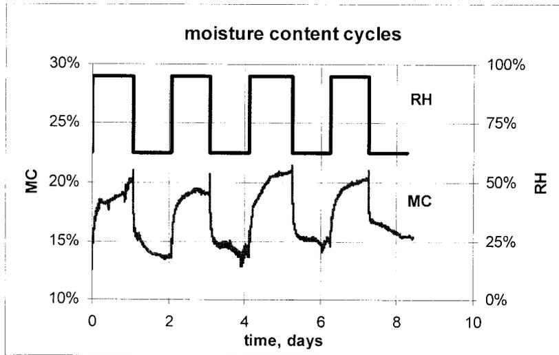
FIG. 4. Relative humidity (RH) and the specimens moisture content (MC) cycles in the free swelling/shrinkage test.
