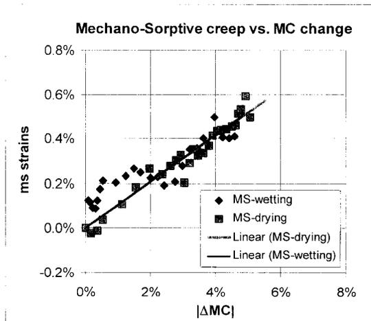
FIG. 8. Mechano-sorptive creep vs. absolute change in MC.
