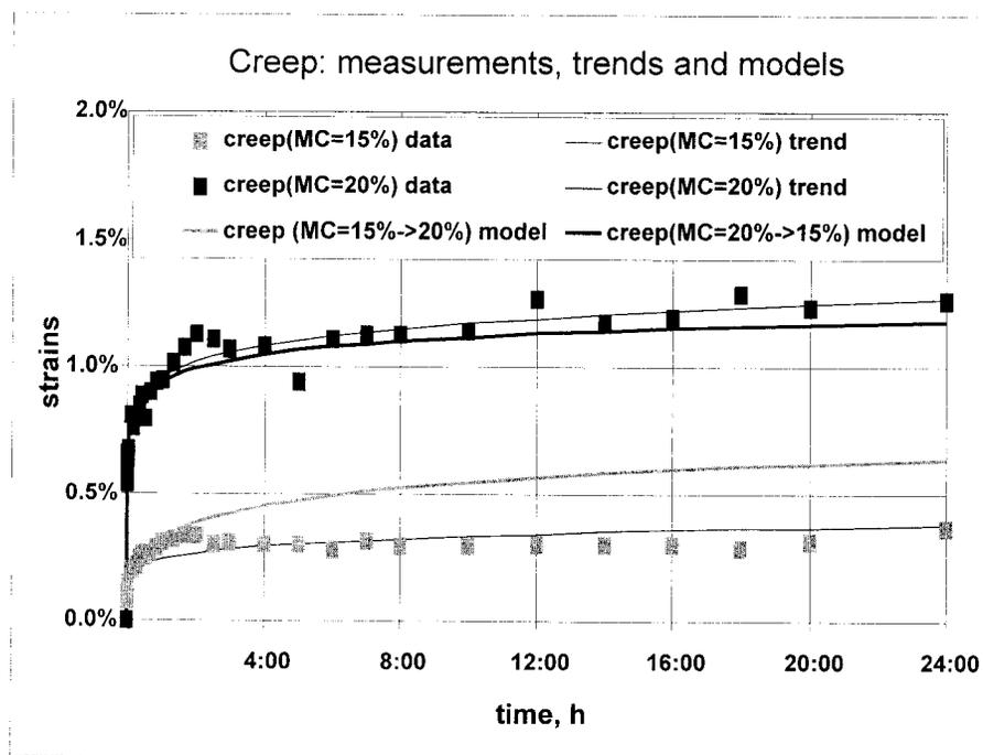
FIG. 6. Viscoelastic creep components of the total deformation: strain data acquired from the experiment for stable wet and dry conditions (gray square and black square), model curves for stable conditions (thin solid gray line and thin solid black line), and model curves for changing MC (thick solid gray line and thick solid black line).
