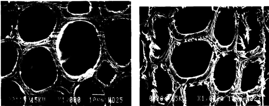
FIG. 2. Transverse face of modern (A) and ancient (B) kauri (*Agathis australis*), showing the rounded to irregularly polygonal tracheids of the earlywood bordered by large intercellular spaces. Band = 10  $\mu\text{m}$ .
