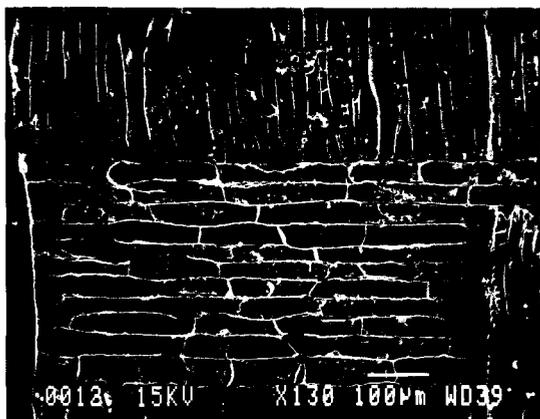
FIG. 5. Radial longitudinal face of carbon-coated ancient kauri (*Agathis australis*). EDS scans of the particles within the rays indicated a sulfur-rich material. These particles were absent in the modern kauri wood. Sulfur compounds are abundant in swamp environments. Band = 100  $\mu\text{m}$ .
