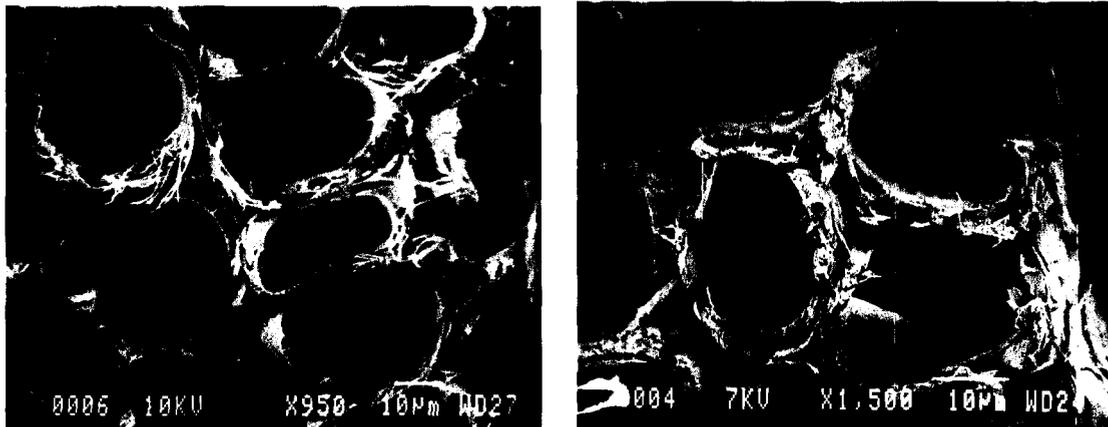
FIG. 7. Transverse fracture surface of the modern (A) and ancient (B) kauri (*Agathis australis*). The  $S_2$  layer of the modern material fractured cleanly, in contrast to the ragged fracture surface of the ancient wood. Loss of carbohydrates within the wood cell wall has altered the strength properties of the ancient kauri. Band = 10  $\mu\text{m}$ .
