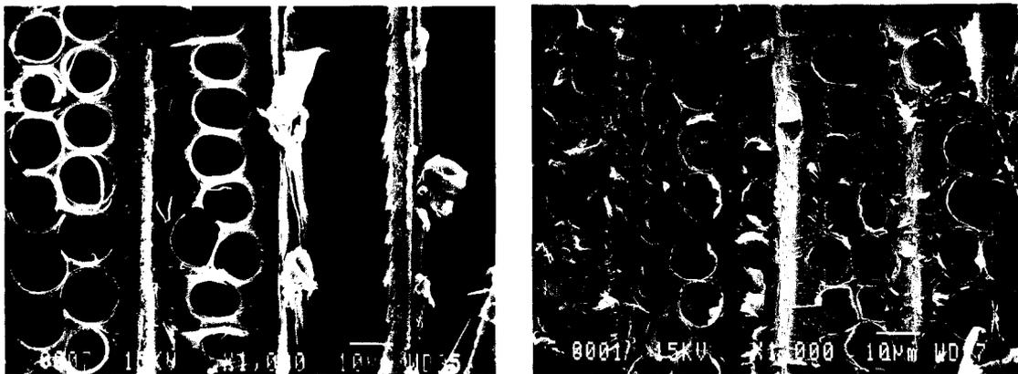
FIG. 3. Radial longitudinal face of modern (A) and ancient (B) kauri (*Agathis australis*). Tori, absent on the intertracheary pits of the modern wood, are visible in the ancient wood. Band = 10  $\mu\text{m}$ .
