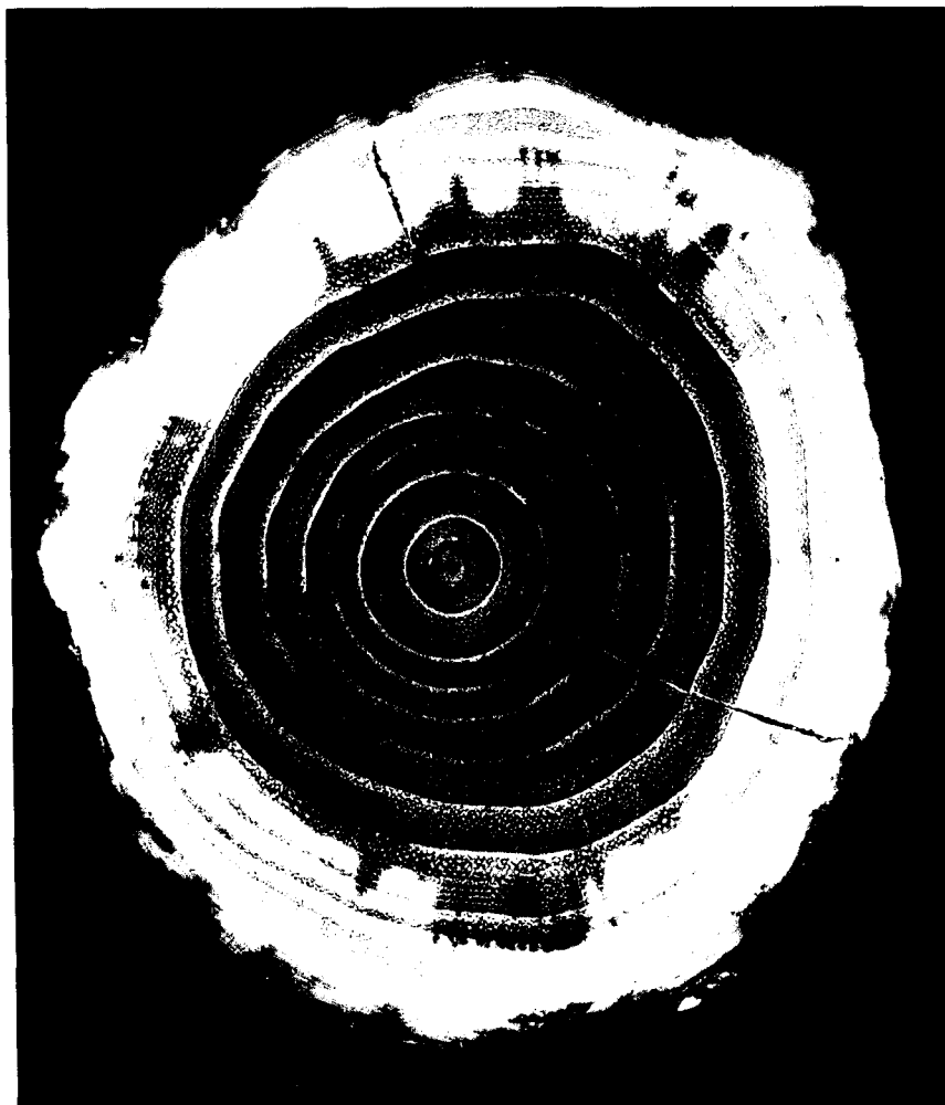
FIG. 2. Typical cross-section of black locust stem-wood showing uneven annular distribution of pigmented extractives.
