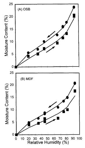
FIG. 1. Typical sorption isotherms for OSB (A) and MDF (B) at  $25^{\circ}$ C. Lines show values predicted by the model.
