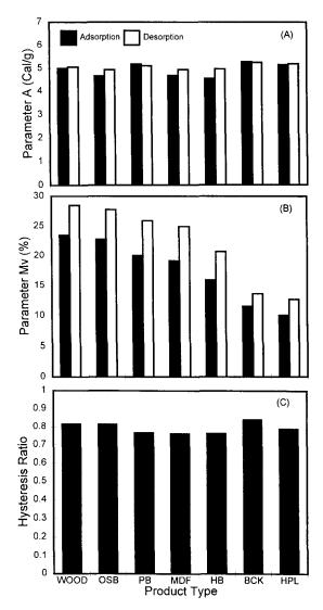
FIG. 2. A comparison of sorption parameters for various materials tested. (A) Parameter A, (B) Parameter my and (C) Hysteresis Ratio.
