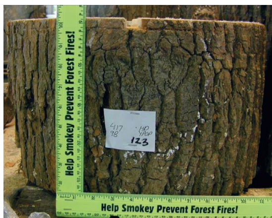
FIG. 2. Defect section with tagged defect and reference groove.
