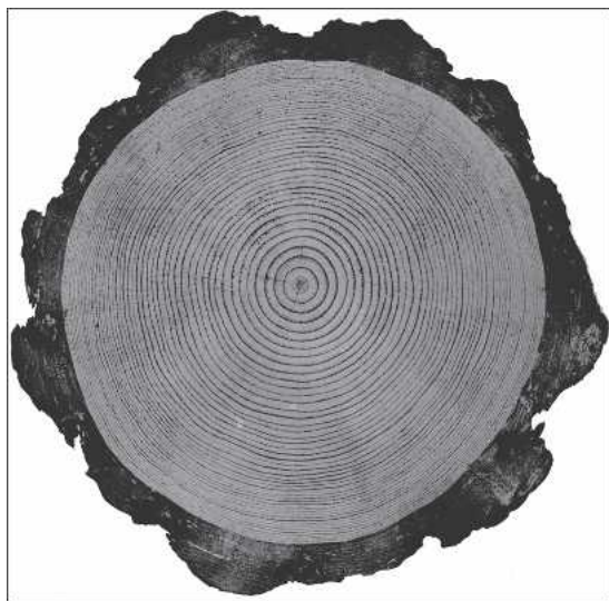
FIG. 1. Cross-section of ponderosa pine log showing growth rings: light bands are earlywood, dark bands latewood.
