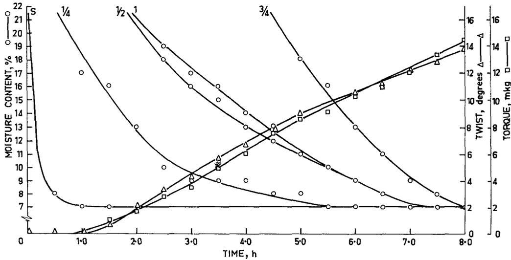
FIG. 2. Moisture contents (%) on the surfaces and at depths of  $\frac{1}{4}$ ,  $\frac{1}{2}$ ,  $\frac{3}{4}$  and 1 inch, twist (degrees), and torque (m kg) measured over the first 8 hr of unrestrained high-temperature drying of test sample no. 1B.
