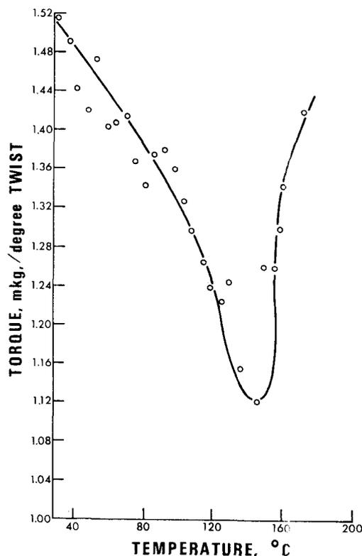
FIG. 3. Effect of increasing temperature on torque (m kg) per degree twist developed in a dry test sample no. 33B.
