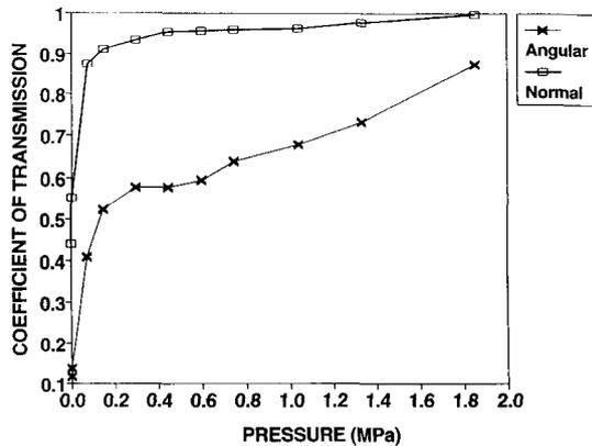
FIG. 5. Effect of pressure on relative coefficient of transmission ( $CT_{rel}$ ) for angular and normal transmission for a kissing bond.
