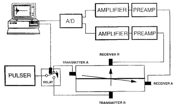
FIG. 2. Curing monitor signal flowchart with a nominal specimen.
