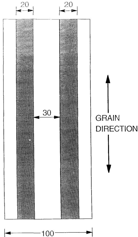
FIG. 3. Uneven bond line spread, showing the adhesive in shadowed areas (top view of the bond line plane) (mm).
