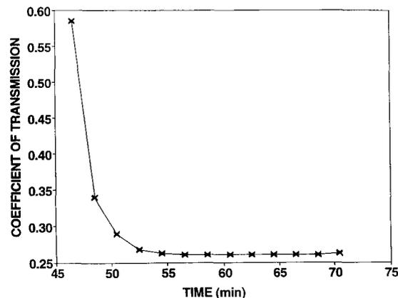
FIG. 6. Unloading effect for kissing bonds [relative coefficient of transmission for angular incidence ( $CT_{rel}^A$ ) vs. curing time], showing time-dependent behavior after removal of the clamping load. Time  $t = 0$  corresponds to the start of loading.
