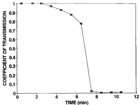
FIG. 7. Relative coefficient of transmission for angular incidence ( $CT_{rel}^A$ ) for a kissing bond under tension, showing time-dependent behavior and abrupt drop of  $CT_{rel}^A$  caused by the bond separation.
