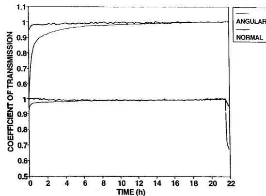
FIG. 4. Typical curing curve (relative coefficient of transmission vs. curing time) for normal bonds (upper curves) and kissing bonds (lower curves).
