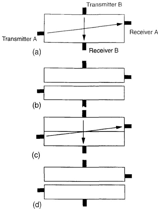
FIG. 1. Specimens with attached transducers in different testing phases: (a) transmission through a solid specimen without an adhesive bond line, (b) the specimen after sawing and planing, (c) transmission through the laminated specimen with an adhesive bond line, and (d) the resawn specimen after the first curing monitoring test, prepared for the next testing cycle.
