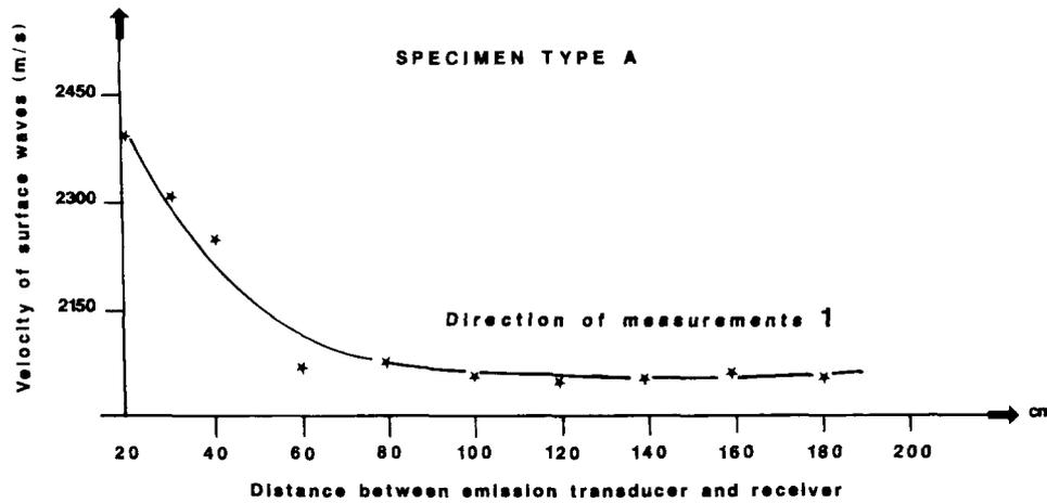
FIG. 4. Variation of surface velocity versus measurement distance.
