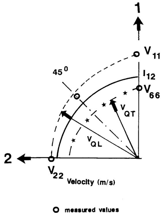
FIG. 3. Velocity surface in the 1,2 plane.
