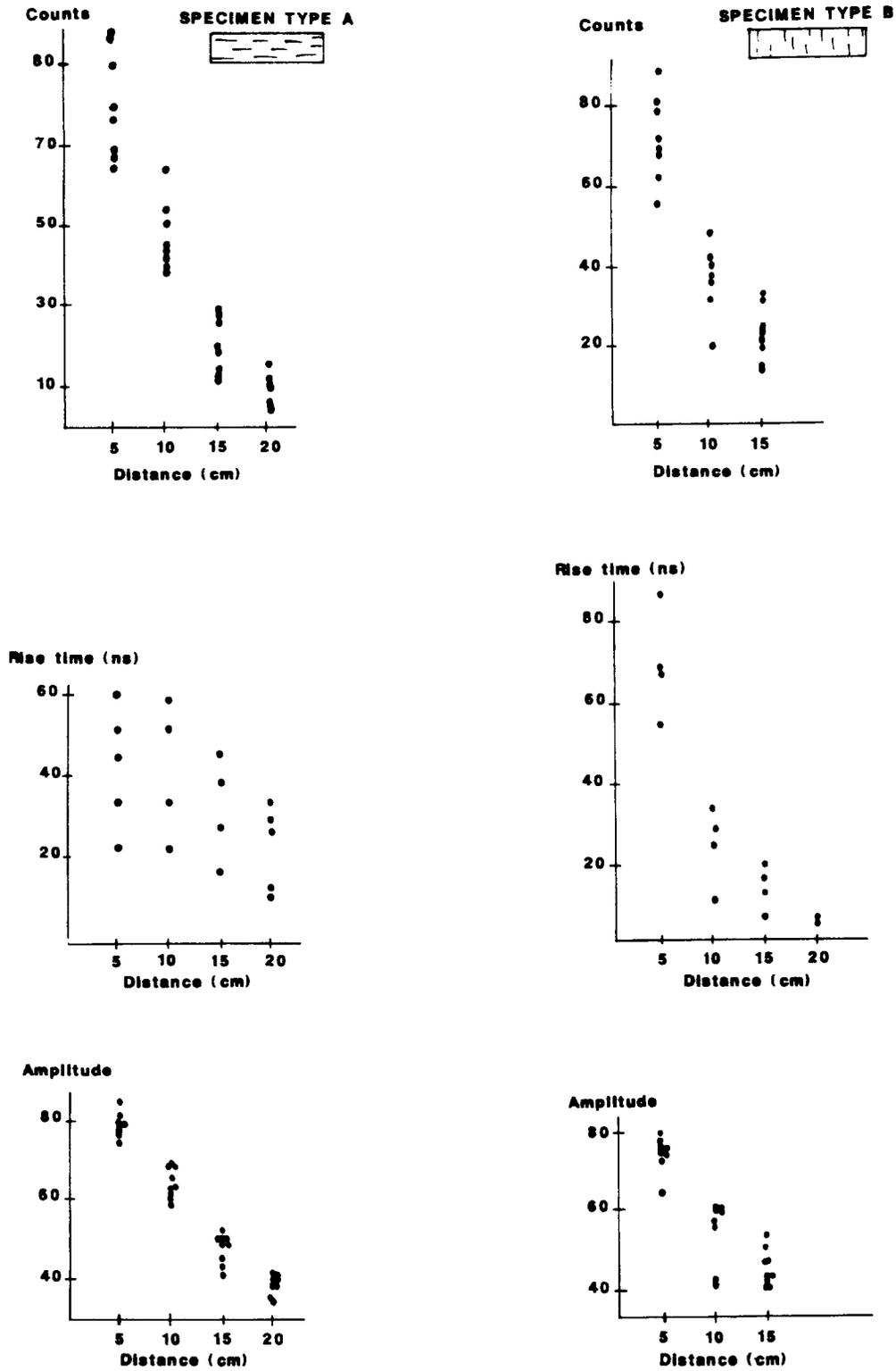
FIG. 5. Acoustic emission parameters measured on Type A and Type B specimens.
