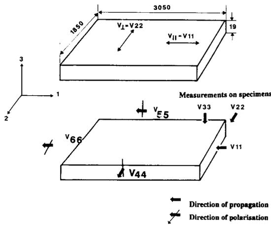
FIG. 1. Velocity measurements on board and specimens.
