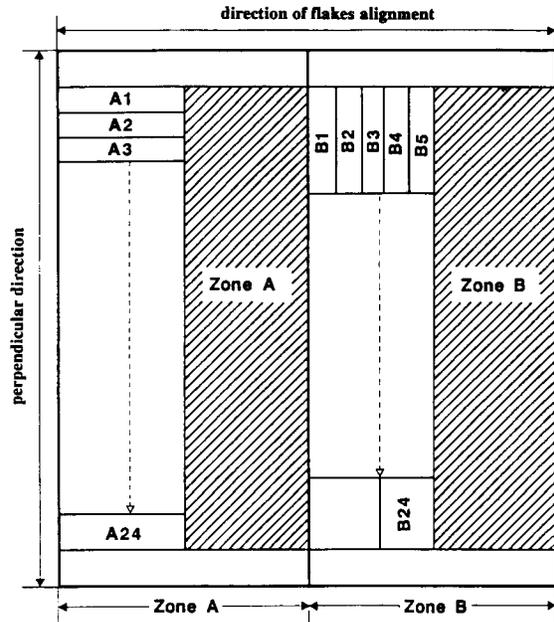
FIG. 2. Sampling strategy. Specimens Type A were cut parallel to the direction of the flake alignment and the specimens Type B were cut perpendicular.
