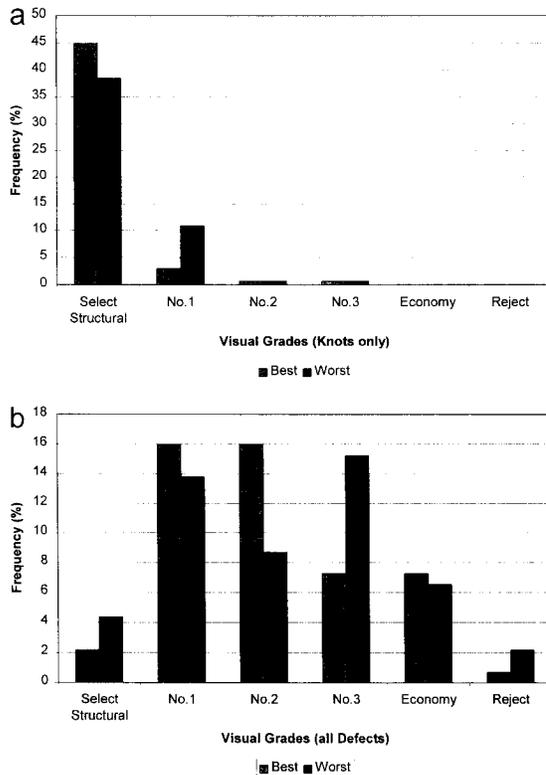
FIG. 6. A) Frequency distribution between best and worst solutions for grading by knots only and B) when all defects are considered.
