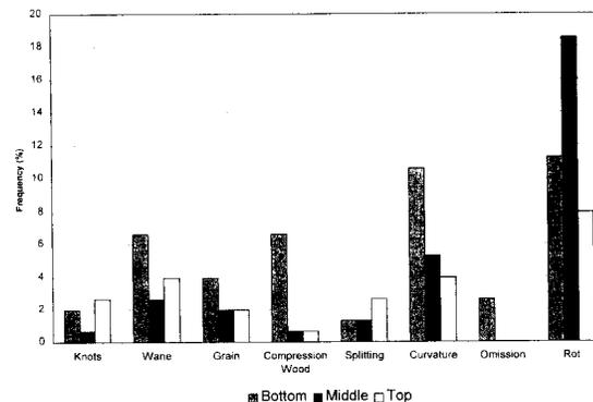
FIG. 5. Impact of the various defects in the overall grade of the boards.
