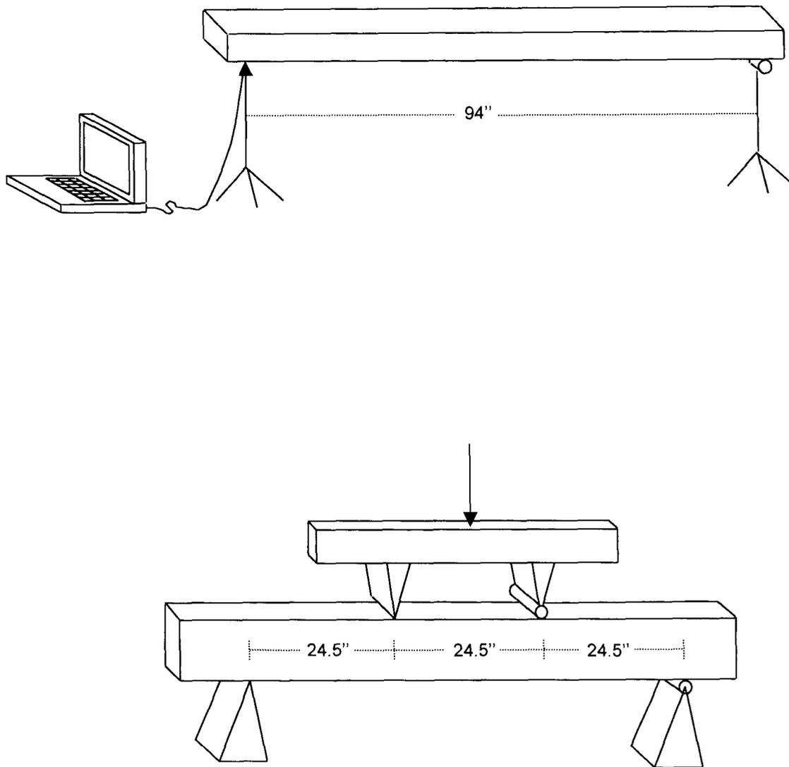
FIG. 3. A) Testing the boards using an e-computer. B) Standard third point bending test for the boards.
