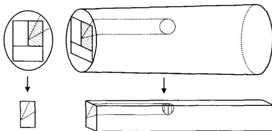
FIG. 1. Sawing pattern used to mark the small end of logs.
