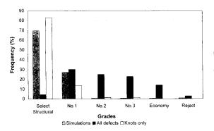
FIG. 4. Distribution of grades—comparison among simulations, actual board grades (knots only) and grades (all defects) based on board grade output.
