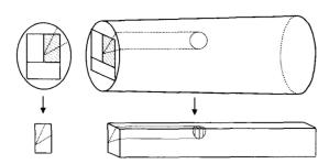
FIG. 1. Sawing pattern used to mark the small end of logs.
