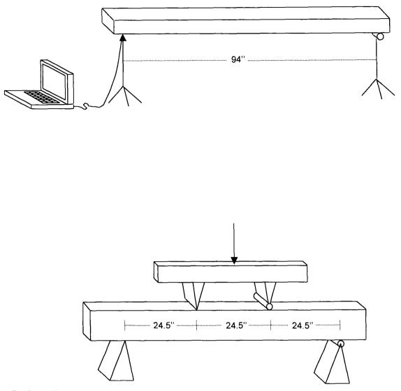
FIG. 3. A) Testing the boards using an e-computer. B) Standard third point bending test for the boards.
