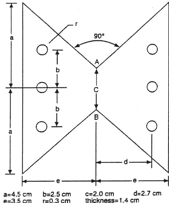
Fig. 2 Geometric dimensions of specimen.
