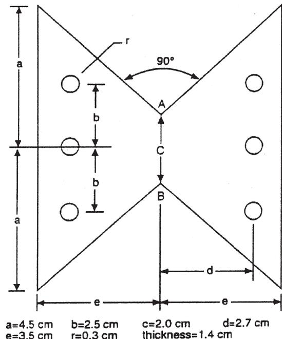
Fig. 2 Geometric dimensions of specimen.
