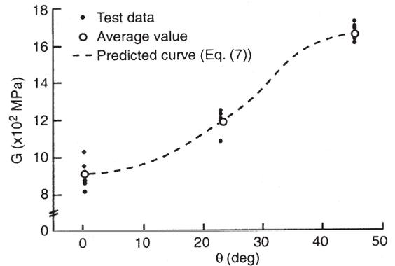
Fig. 3 Variation of shear modulus  $G$  with grain slope  $\theta$
