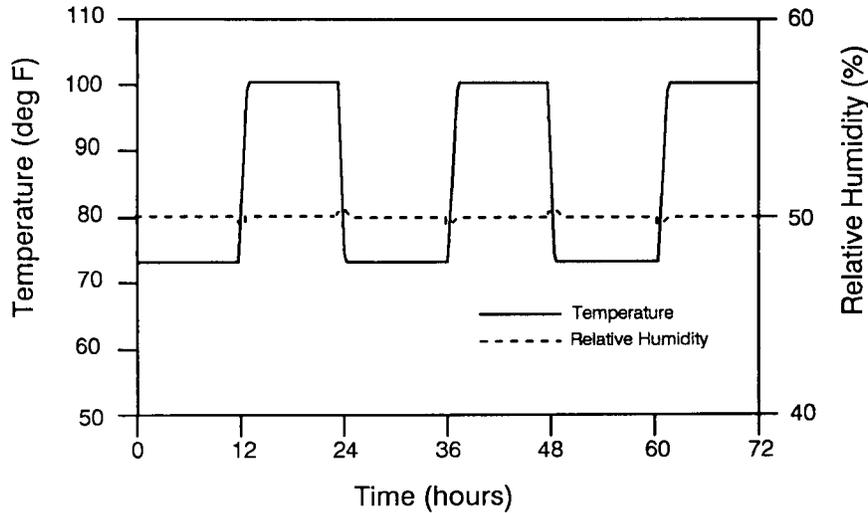
FIG. 1. Imposed 73-100 F temperature cycle.
