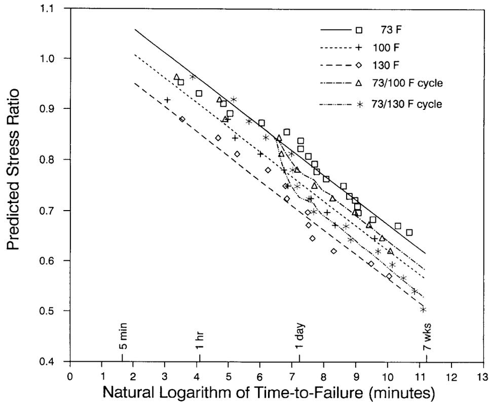
FIG. 6. Relationship between predicted stress ratio and the natural logarithm of time-to-failure for No. 2 lumber.
