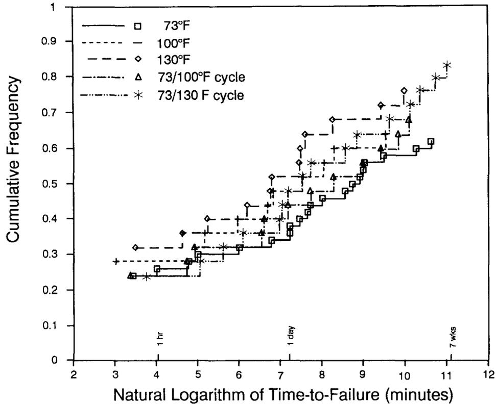
FIG. 4. Cumulative frequency distribution of times-to-failure for No. 2 lumber.
