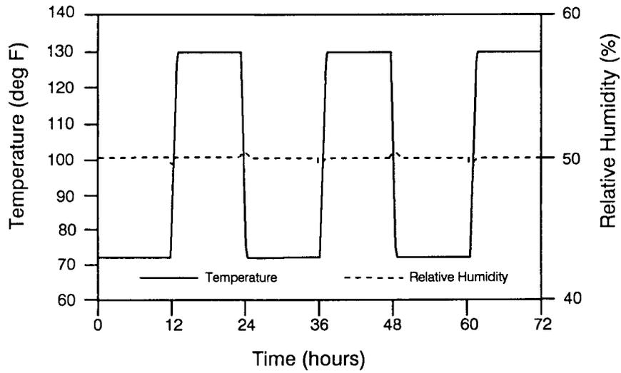
FIG. 2. Imposed 73-130 F temperature cycle.
