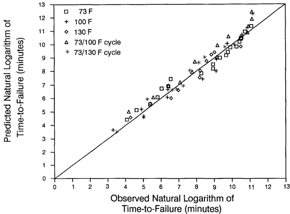
FIG. 7. Relationship between predicted and observed natural logarithm of time-to-failure for Select Structural lumber.
