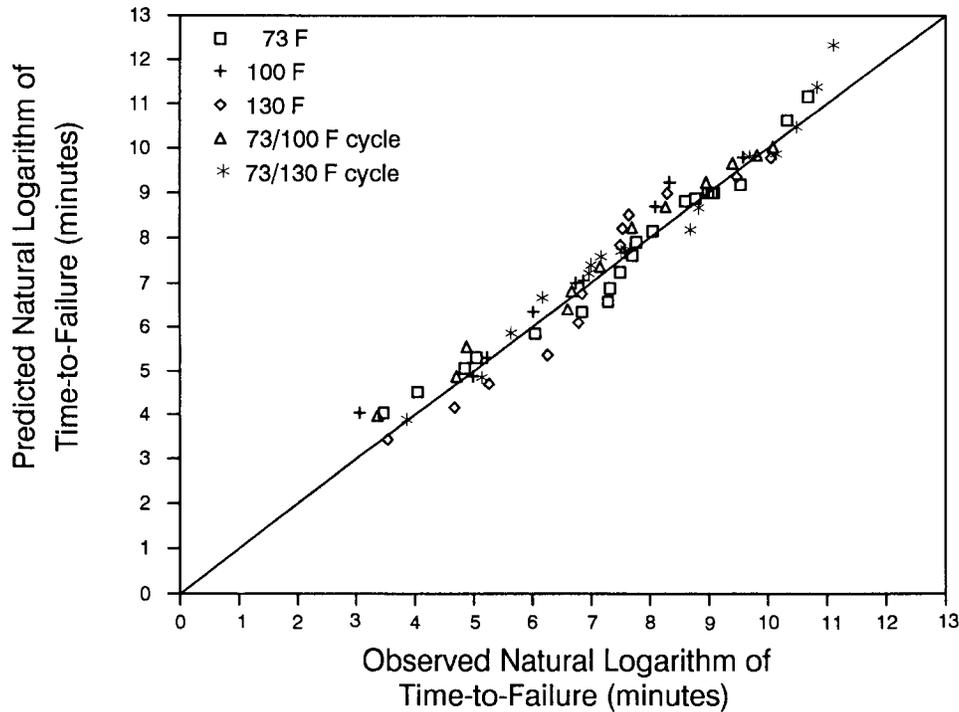
FIG. 8. Relationship between predicted and observed natural logarithm of time-to-failure for No. 2 lumber.
