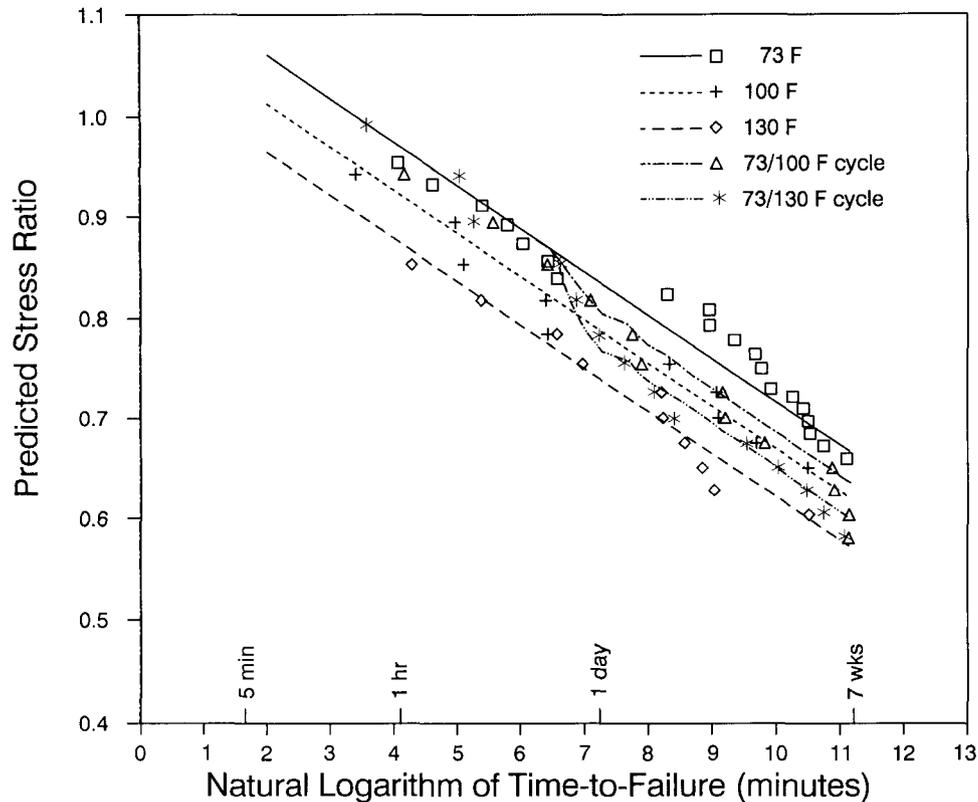
FIG. 5. Relationship between predicted stress ratio and the natural logarithm of time-to-failure for Select Structural lumber.
