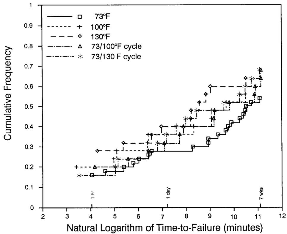
FIG. 3. Cumulative frequency distribution of times-to-failure for Select Structural lumber.
