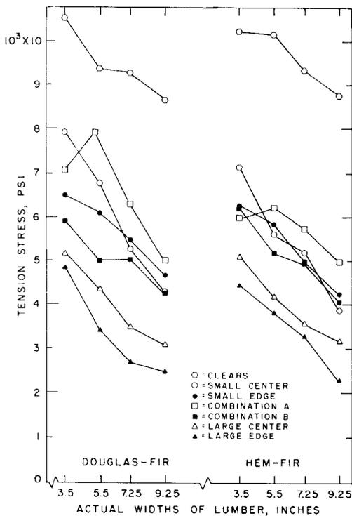
FIG. 5. Average values of tension stress for the various categories of knots for Douglas-fir and hem-fir 2-inch dimension lumber of nominal 4-, 6-, 8-, and 10-inch widths. Douglas-fir was at 9 and hem-fir at 10% moisture content when tested. Plotted points are an average of 22 specimens except for the large center knot samples, which had fewer specimens (see Table 1).
