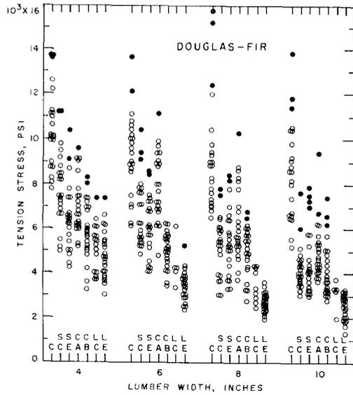
FIG. 3. Distributions of tension stress obtained from tests of nominal 2- by 4-, 6-, 8-, and 10-inch Douglas-fir dimension lumber at 9% moisture content. Code for samples: C for clears, SC for small center, SE for small edge, CA and CB for knot combinations A and B, LC for large center, and LE for large edge knots. See Table 1 for sizes of knots in the different samples within each size of lumber. Solid circles were the values excluded so that remaining values were the adjusted distributions.
