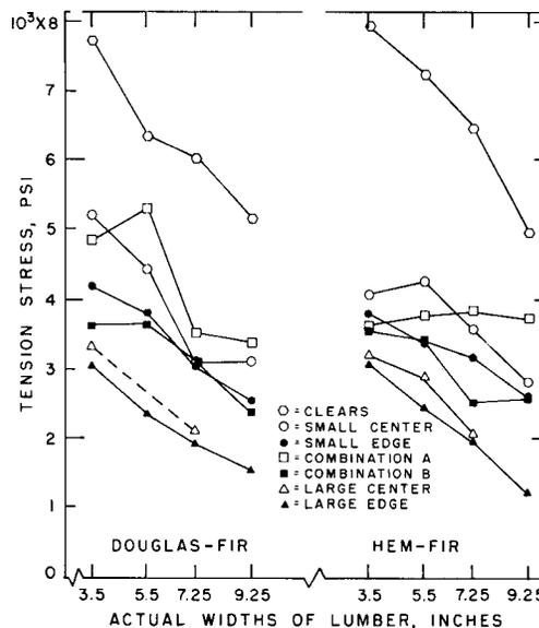
FIG. 6. Tension stress values at the lower 5% exclusion limit for the various categories of knots for Douglas-fir and hem-fir 2-inch dimension lumber of nominal 4-, 6-, 8-, and 10-inch widths. Douglas-fir was at 9 and hem-fir at 10% moisture content when tested. Plotted points were calculated from the adjusted distributions in which some of the greater test values were not included. See Figures 1-4 for values left out.
