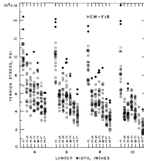
FIG. 4. Distributions of tension stress obtained from tests of nominal 2- by 4-, 6-, 8-, and 10-inch hem-fir dimension lumber at 10% moisture content. Code for samples: C for clears, SC for small center, SE for small edge, CA and CB for knot combinations A and B, LC for large center, and LE for large edge knots. See Table 1 for sizes of knots in the different samples within each size of lumber. Solid circles were the values excluded so that remaining values were the adjusted distributions.
