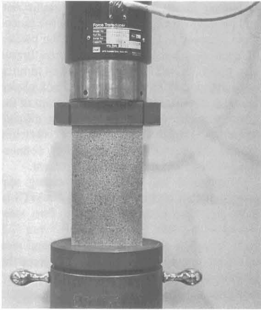
FIG. 2. Photograph displaying the aluminum block evaluation test setup.
