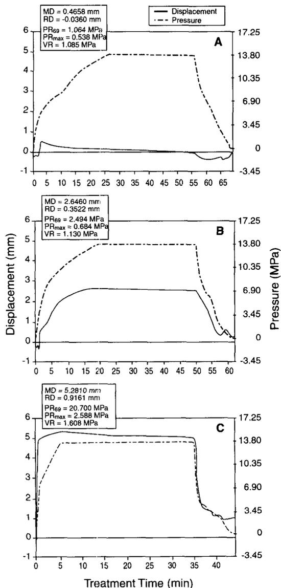
FIG. 2. Effect of rate of pressurization on deformation of white spruce lumber during supercritical fluid impregnation where the target rate of pressurization is (A) 1.035 MPa/min, (B) 2.332 MPa/min, and (C) 19.769 MPa/min. MD = maximum displacement, RD = residual displacement,  $PR_{6.9}$  = pressurization rate to 6.9 MPa,  $PR_{max}$  = maximum pressurization, and VR = venting rate.
