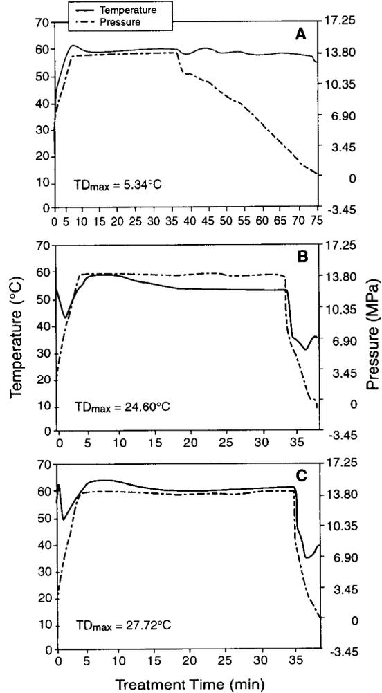
FIG. 4. Wood temperature during supercritical fluid impregnation when samples are pressurized to 13.8 MPa at a rate between 2.905 and 4.092 MPa/min at an initial temperature of 60°C, held for 30 min, and then vented at (A) 0.359 MPa/min, (B) 2.560 MPa/min, and (C) 3.788 MPa/min. TD<sub>max</sub> = maximum temperature drop during ventilation.
