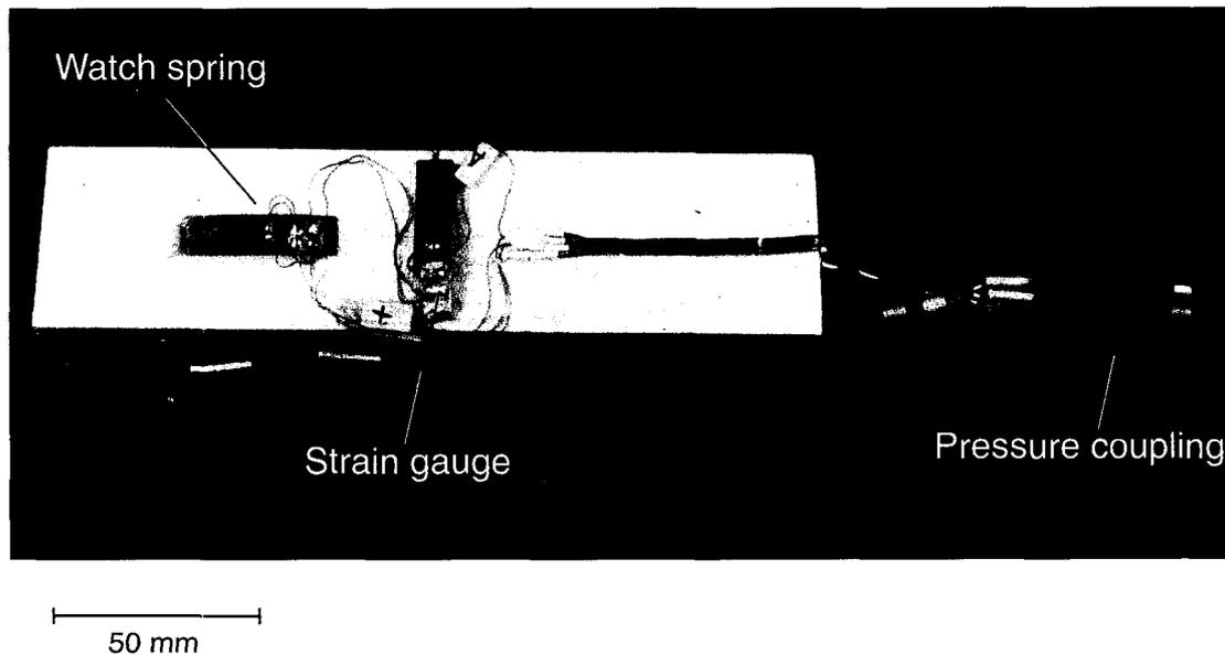
FIG. 1. System used to measure displacement on spruce wood during supercritical fluid impregnation with carbon dioxide.
