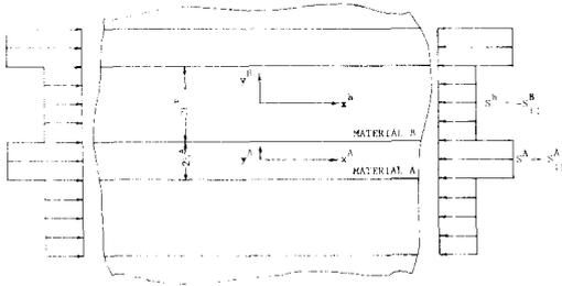
FIG. 1. Layered medium subjected to a state of initial homogeneous strain.
