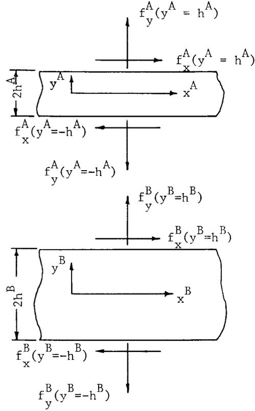
FIG. 2. Boundary stresses at the interfaces between layers.
