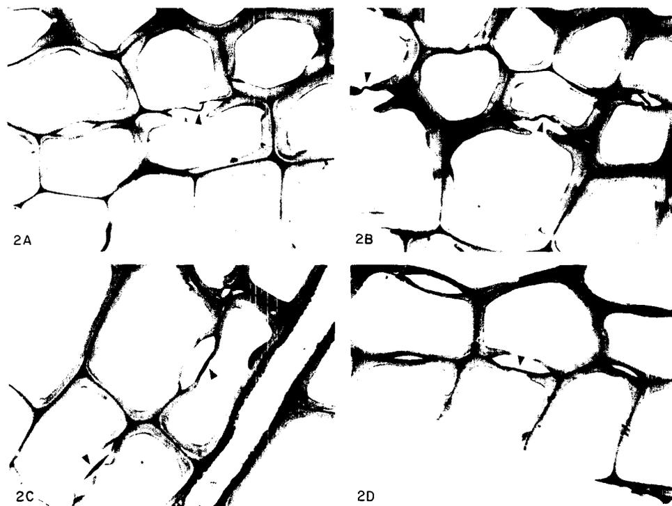
FIG. 2. A. Unextracted heartwood cross section. Torus (arrows). Freeze-sectioned. UV micrograph.  $w_m = 90 \mu\text{m}$ . B. Extracted heartwood cross section. Tori (arrows). Freeze-sectioned. UV micrograph.  $w_m = 90 \mu\text{m}$ . C. Unextracted heartwood cross section. Tori (arrows). Epon embedded. UV micrograph.  $w_m = 90 \mu\text{m}$ . D. Extracted heartwood cross section. Torus (arrow). Epon embedded. UV micrograph.  $w_m = 90 \mu\text{m}$ .
