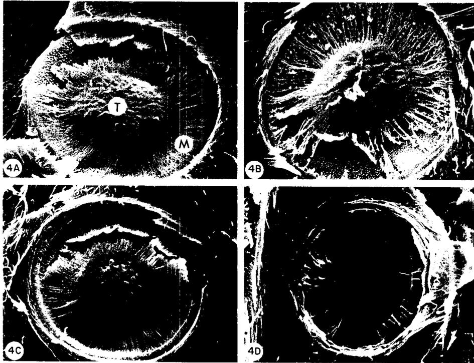
FIG. 4. A. Bordered pit torus (T) and margo region (M). Unextracted sapwood. Critical-point dried (CPD). Scanning electron micrograph (SEM).  $w_m = 25 \mu\text{m}$ . B. Bordered pit torus and margo region. Extracted sapwood. CPD. SEM.  $w_m = 25 \mu\text{m}$ . C. Bordered pit torus and margo region. Unextracted heartwood. CPD. SEM.  $w_m = 25 \mu\text{m}$ . D. Bordered pit torus and margo region. Extracted heartwood. CPD. SEM.  $w_m = 25 \mu\text{m}$ .
