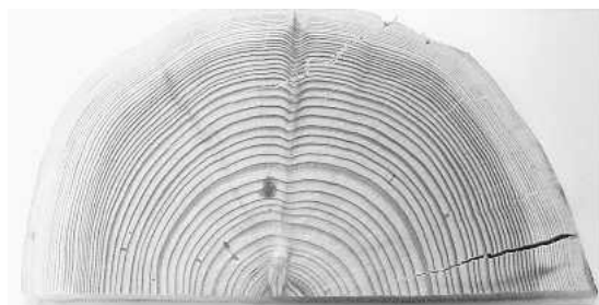
FIGURE 1. The picture of the wood disk used in this study. All measurements were conducted on the right half of the wood core sample (2 mm in tangential direction) cut from the bottom.
