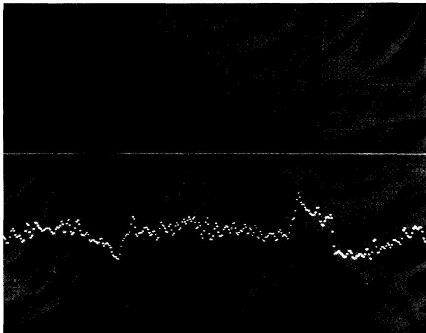
FIG. 7. Cl line scan, Cellon-treated specimen. 400-second analysis; 1000 $\times$ ; 40 $^\circ$  tilt.
