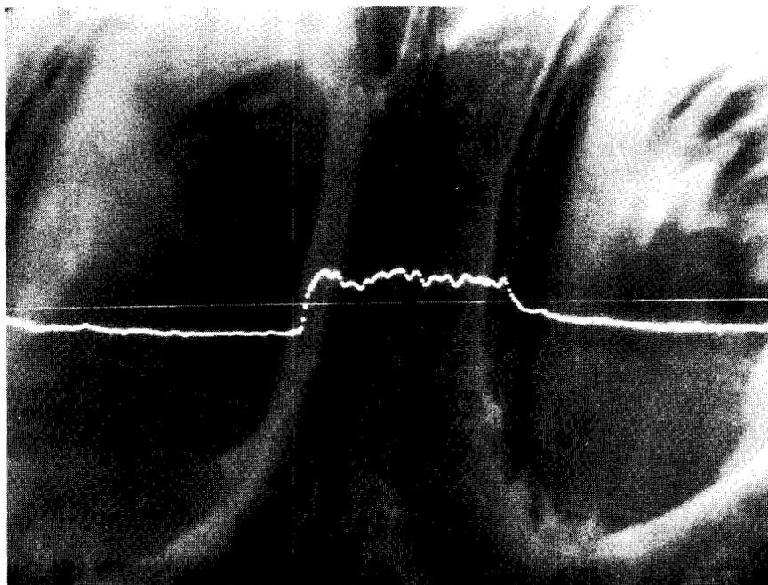
FIG. 9. Cl line scan, benzene-extracted PCP-PO treatment. 400-second analysis; 2400 $\times$ ; 40 $^\circ$  tilt.
