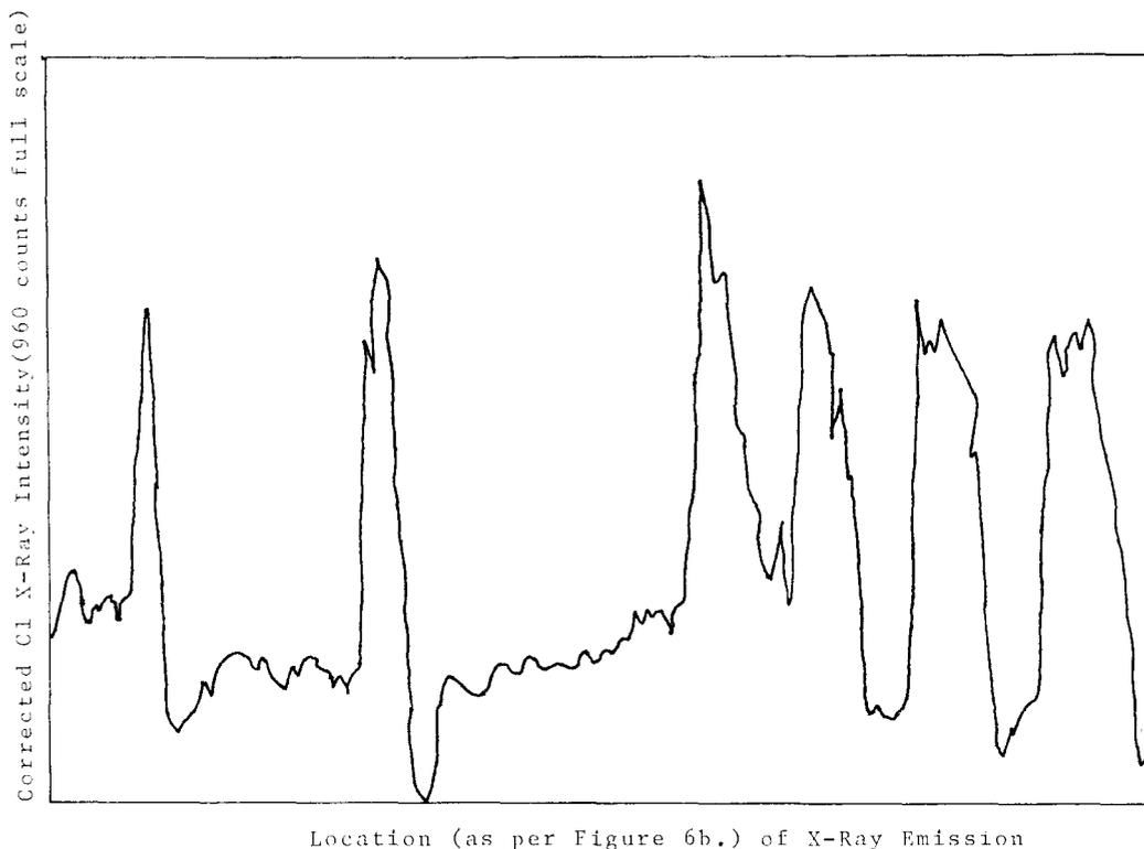
FIG. 6A. Corrected Cl line scan for benzene-extracted, Cellon-treated specimen shown in Fig. 6B. 400-second analysis; 570 $\times$ ; 0 $^\circ$  tilt.
