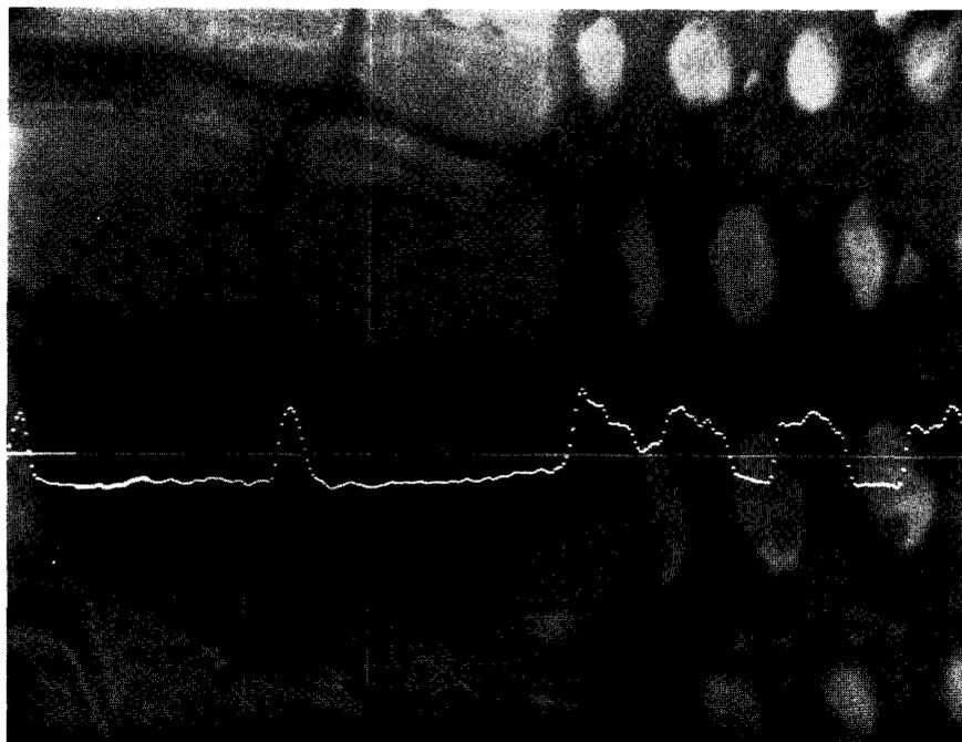
FIG. 6B. Cl line scan, benzene-extracted, Cellon-treated specimen. 400-second analysis; 570 $\times$ ; 0 $^\circ$  tilt.
