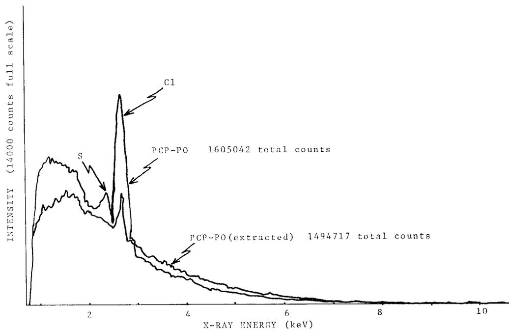
FIG. 8. Energy spectra for (a) PCP-PO treatment, (b) benzene-extracted PCP-PO treatment. 400-second analysis; 220 $\times$ ; 40 $^\circ$  tilt.
