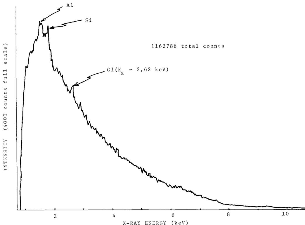
FIG. 1. X-ray energy spectra for control. 600-second analysis; 260 $\times$ ; 0 $^\circ$  tilt angle (all angles are nominal)
