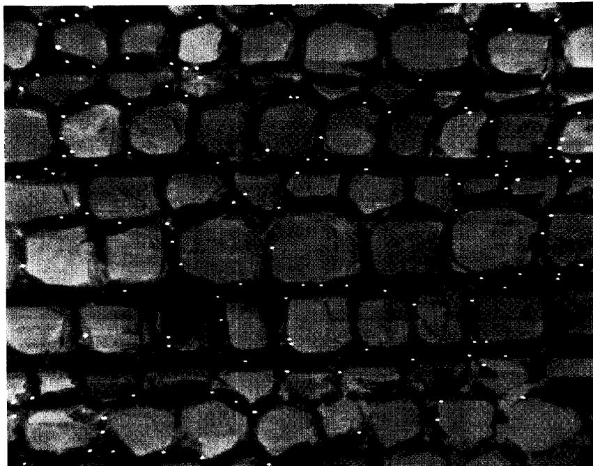
FIG. 2. Element map for Cl control. 600-second analysis; 260 $\times$ ; 0 $^\circ$  tilt angle.
