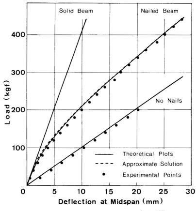
FIG. 6. Typical deflection versus load curves, for D190F.
