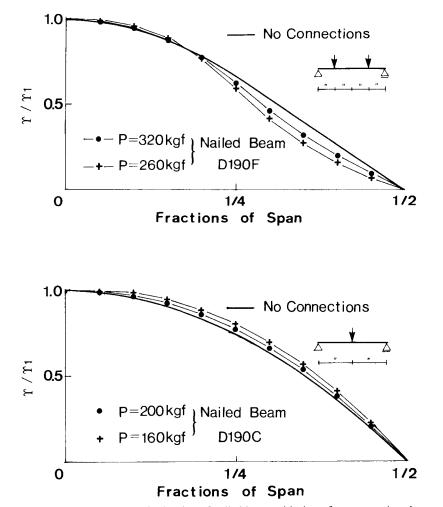
FIG. 4. Comparison of slip distribution of nailed beam with that of no connections beam.
