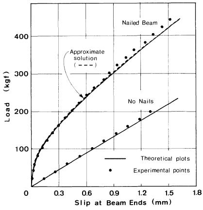
FIG. 8. Typical load versus slip curve at beam ends, for D190F.
