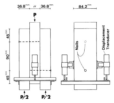
FIG. 5. Nailed joint test.
