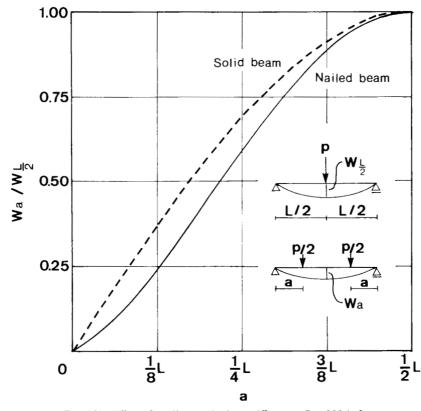
FIG. 12. Effect of loading method on stiffness, at P = 200 kgf.
