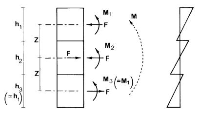
FIG. 3. Three-layer beam forces and strains.
