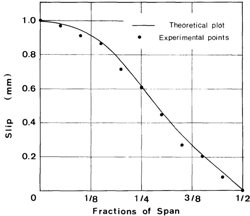
FIG. 9. Typical slip distribution, for D190F at  $P = 320$  kgf.
