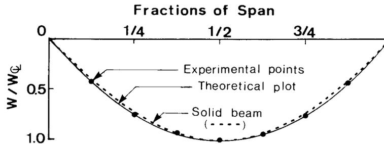
FIG. 7. Typical deflection curve, for D190F at  $P = 200$  kgf.
