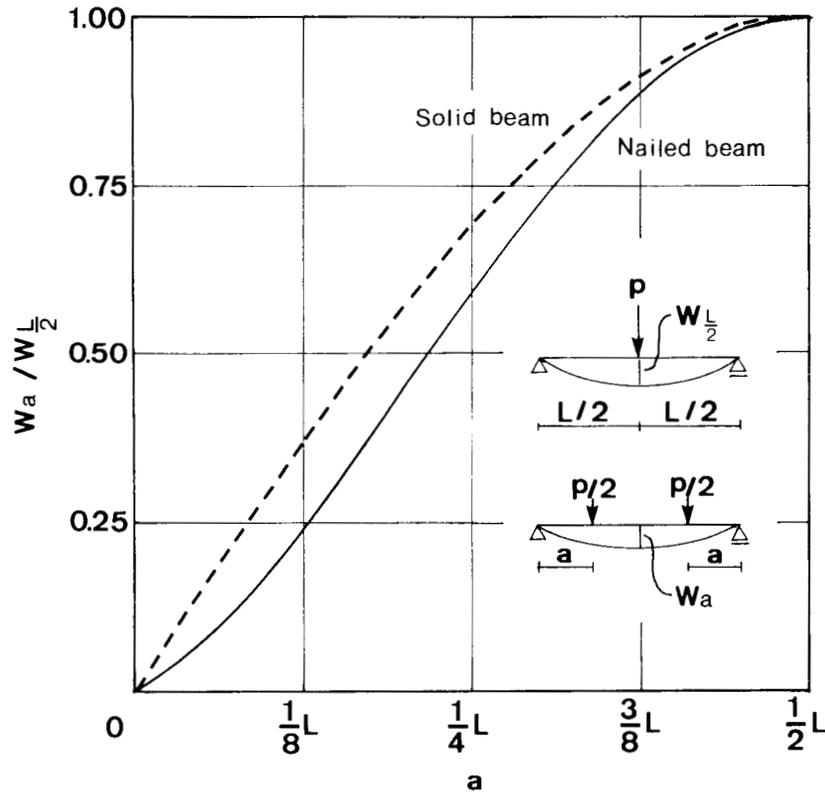
FIG. 12. Effect of loading method on stiffness, at  $P = 200$  kgf.
