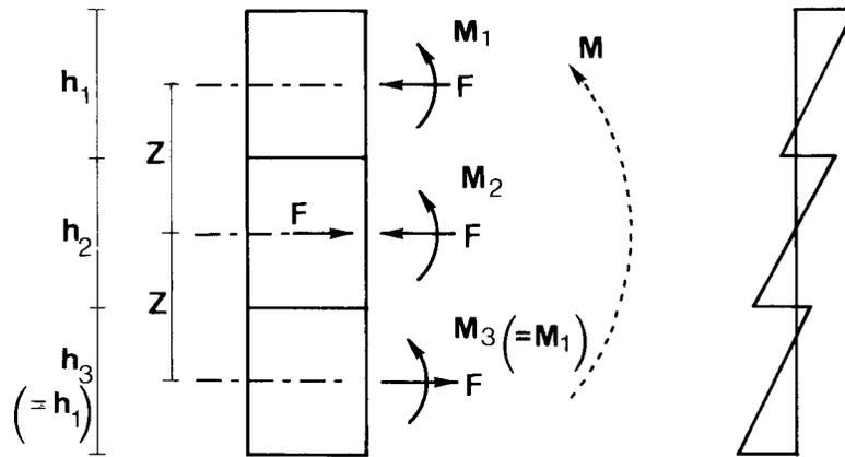
FIG. 3. Three-layer beam forces and strains.
