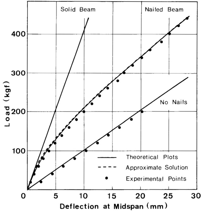
FIG. 6. Typical deflection versus load curves, for D190F.
