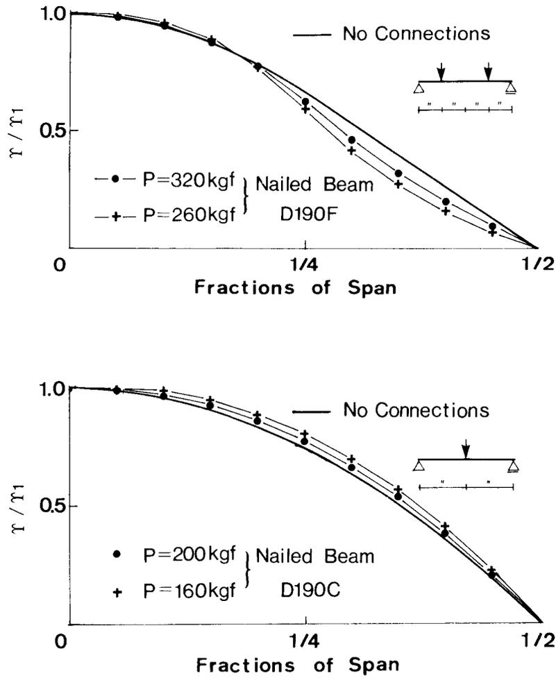
FIG. 4. Comparison of slip distribution of nailed beam with that of no connections beam.
