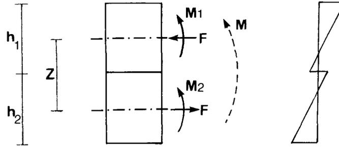
FIG. 1. Two-layer beam forces and strains.
