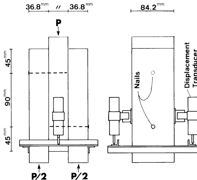
FIG. 5. Nailed joint test.
