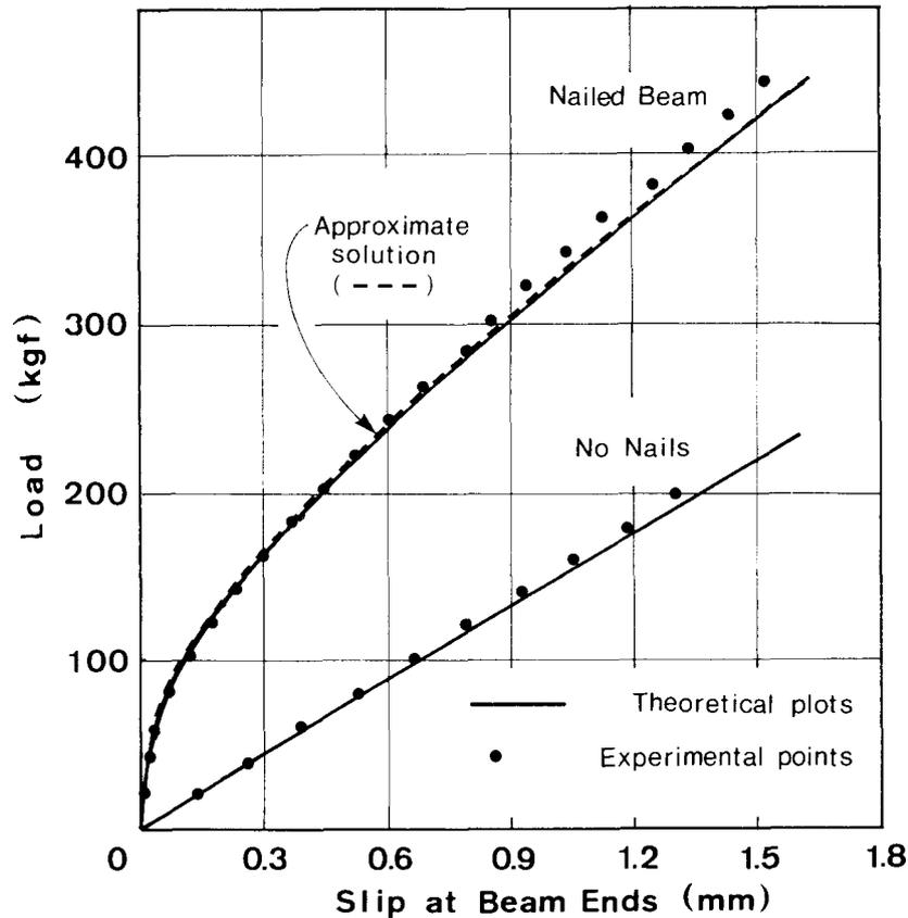
FIG. 8. Typical load versus slip curve at beam ends, for D190F.
