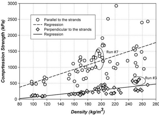
Figure 4. Relationships between density and compression strength in the two loading directions.
