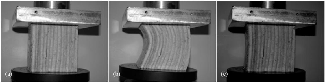
Figure 2. Experimental setup of the compression strength measurements (a) before loading, (b) at maximum load, and (c) at relaxation after unloading.
