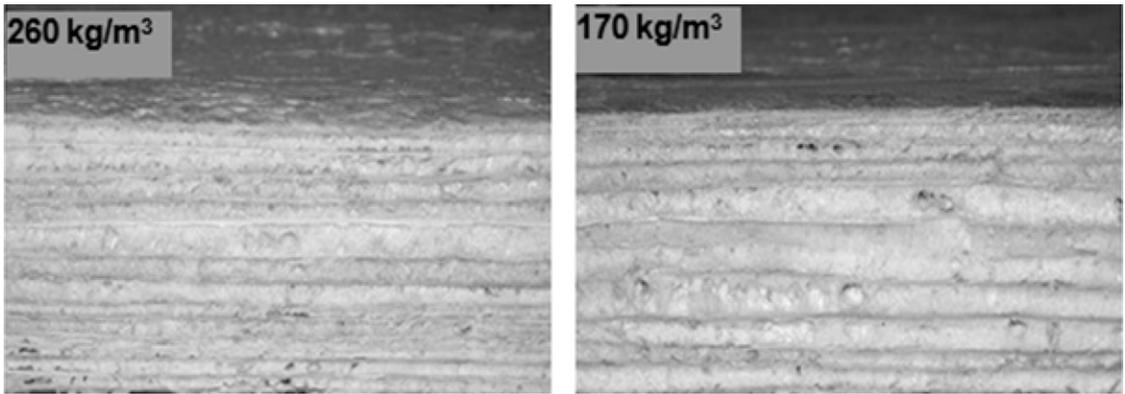
Figure 1. High- and medium-density polyurethane–veneer composites.
