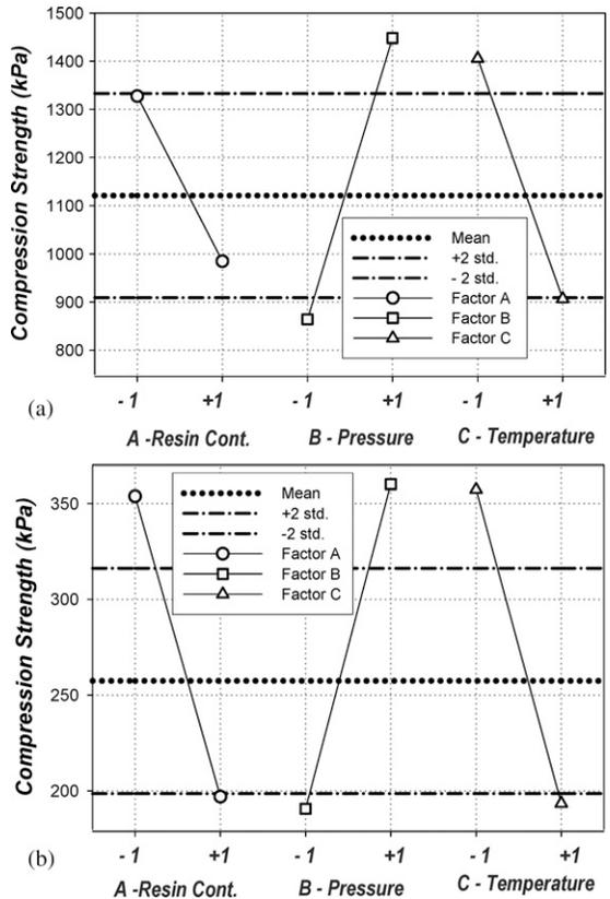
Figure 5. Effects of technological factors on compression strength. (a) Parallel strand alignment and (b) perpendicular strand alignment relative to the direction of applied load.
