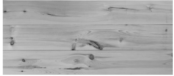
Figure 5. Three characteristic boards from the defect group. (Note large areas of grain deviations.)
