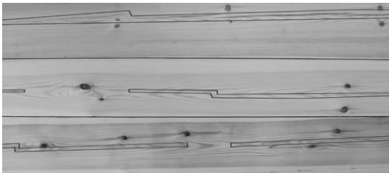
Figure 4. Three characteristic boards from the check group (checks are outlined).
